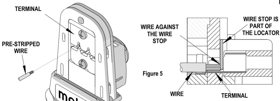
**Note: The tamper proof ratchet action will not release the tool until it has been fully closed.**
