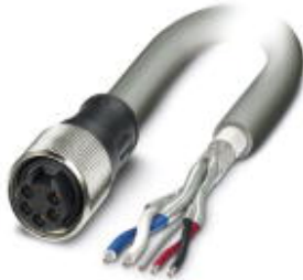
Bus system cable, DeviceNet, 5-position, PVC, Gray RAL 7001, Free cable end, on Socket straight 7/8"-16UNF, Cable length: 5 m
