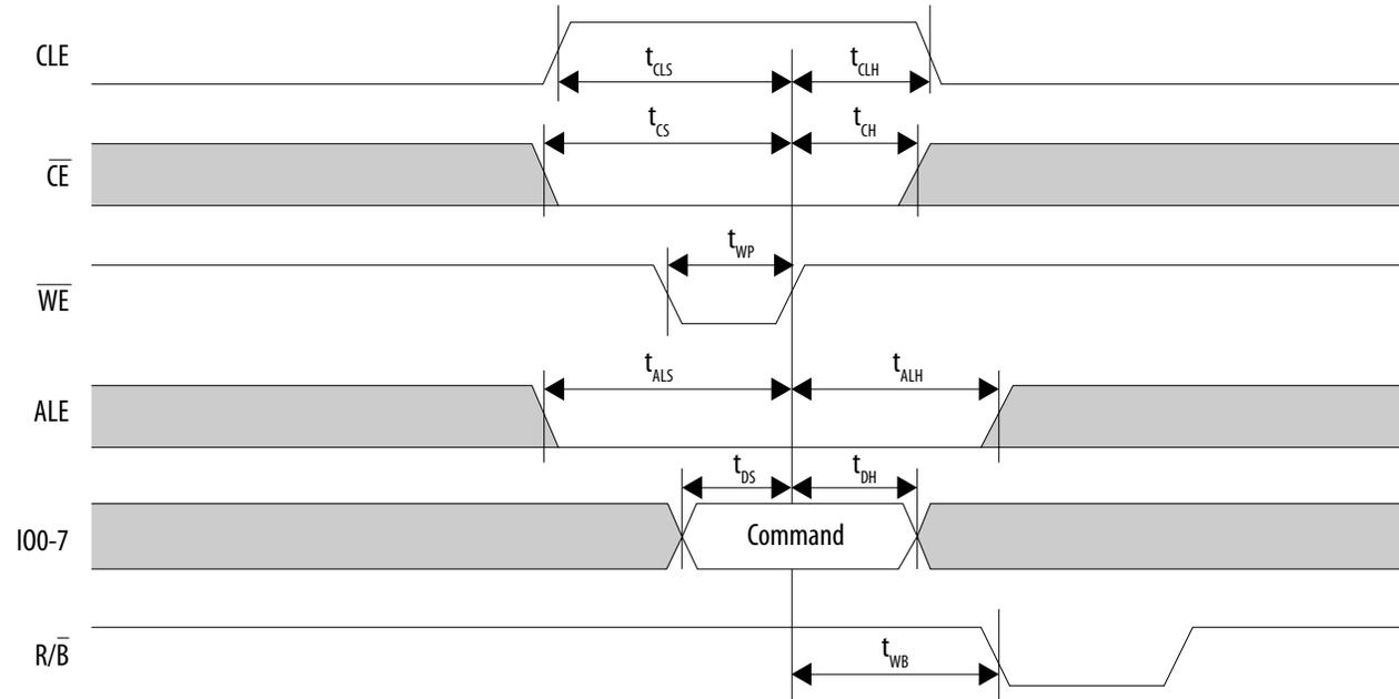
Figure 19. NAND Address Latch Timing Diagram
