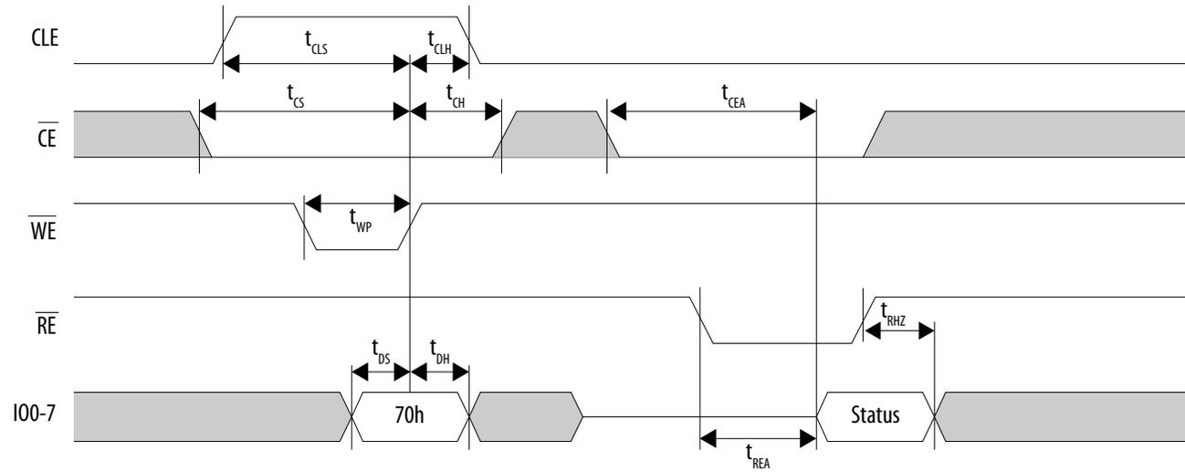
Figure 24. NAND Read Status Enhanced Timing Diagram
