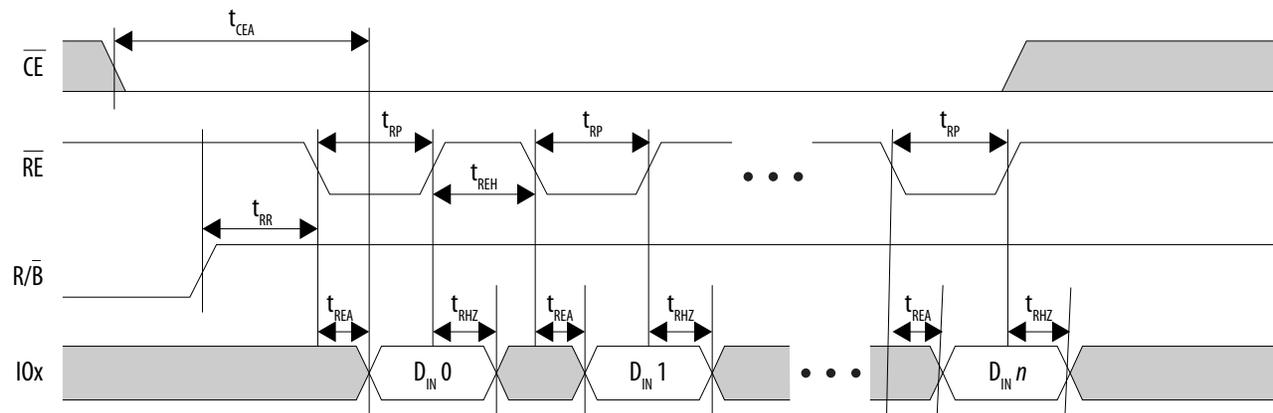
Figure 22. NAND Data Input Timing Diagram for Extended Data Output (EDO) Cycle
