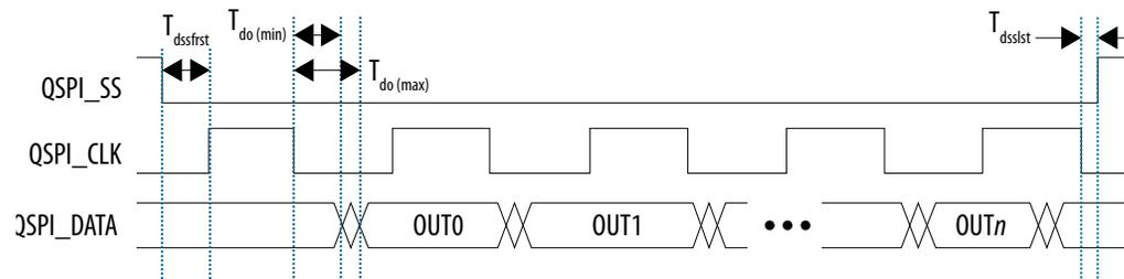
83 This delay is programmable in whole QSPI\_REF\_CLK increments using the `delay` register in the Quad SPI module.
