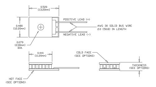
Ceramic Material 96% Alumina Ceramics Solder Construction: 138°C BiSn
