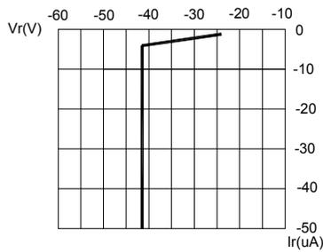
FIG.3 Red & Amber REVERSE CURRENT VS. REVERSE VOLTAGE.
