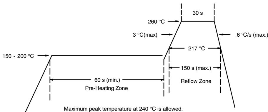
Fig. 4 Solder Reflow Temperatures and Time Durations
