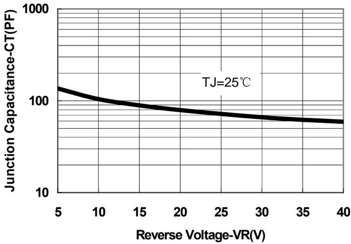
Fig.1-Typical Junction Capacitance
