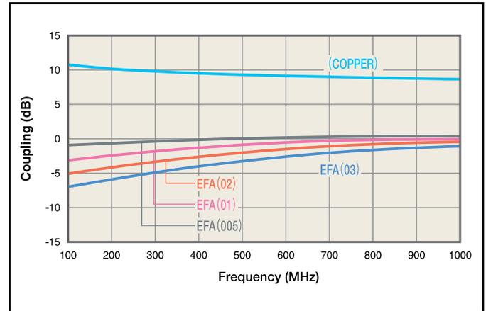
EFH – Attenuation of transmission noise
