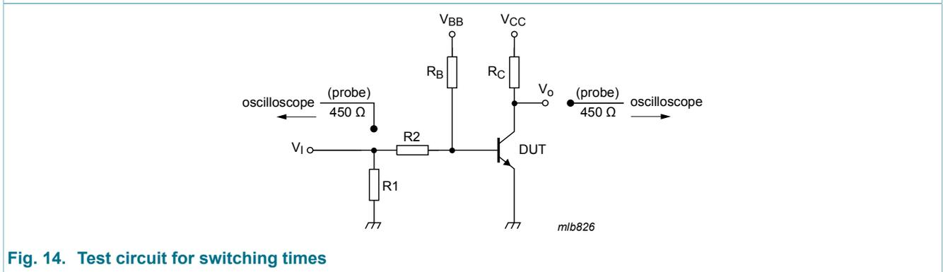
Fig. 14. Test circuit for switching times
