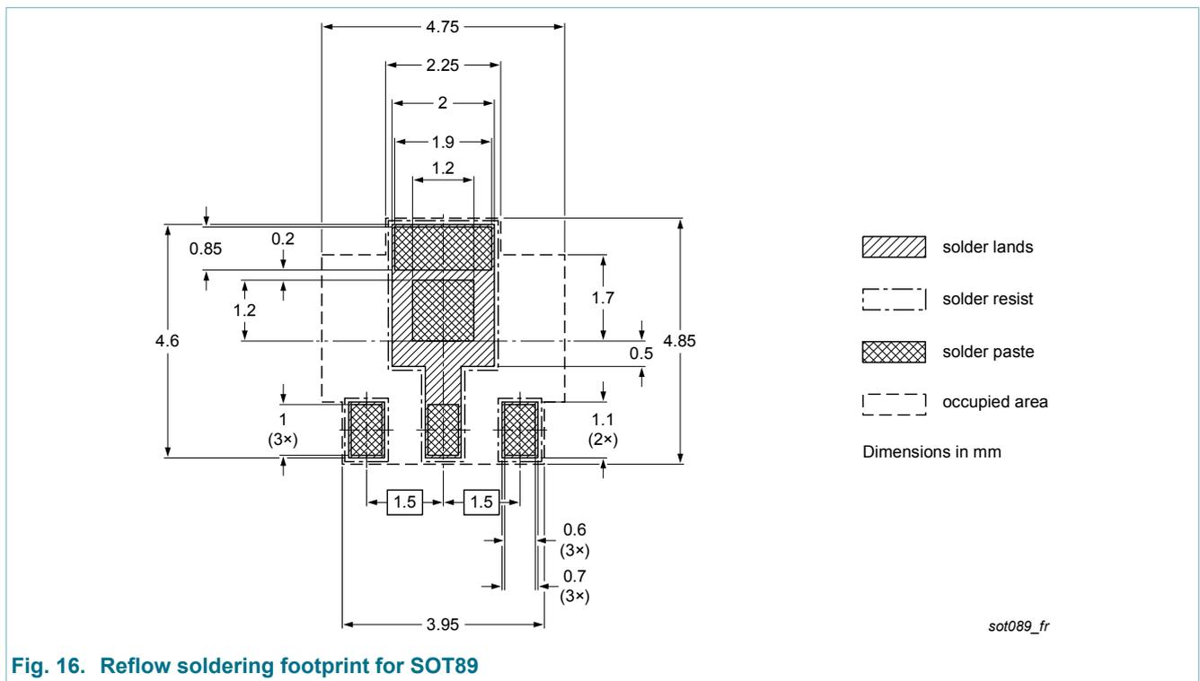
Fig. 16. Reflow soldering footprint for SOT89
