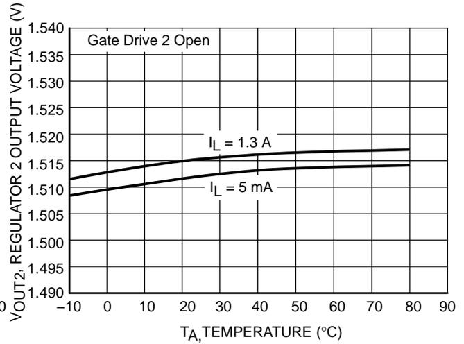
Figure 11. Regulator 2 (Suffix 1) Output Voltage vs. Ambient Temperature
