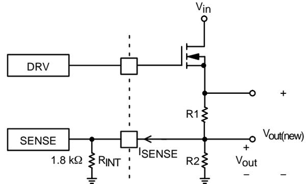
Figure 6. Output Voltage Scaling Using Resistive Network
