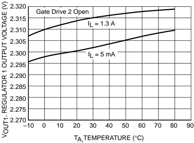
Figure 14. Regulator 1 (Suffix 3) Output Voltage vs. Ambient Temperature
