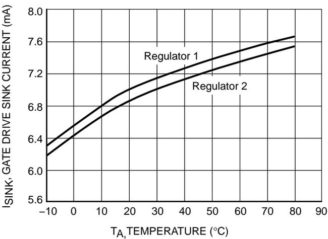
Figure 16. Gate Drive Sink Current vs. Ambient Temperature
