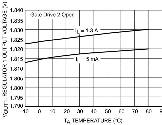
Figure 10. Regulator 1 (Suffix 1) Output Voltage vs. Ambient Temperature
