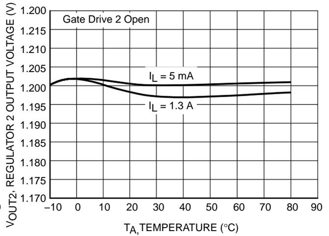
Figure 15. Regulator 2 (Suffix 3) Output Voltage vs. Ambient Temperature
