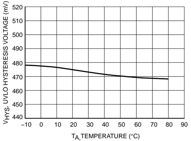
Figure 19. UVLO Hysteresis Voltage vs. Ambient Temperature
