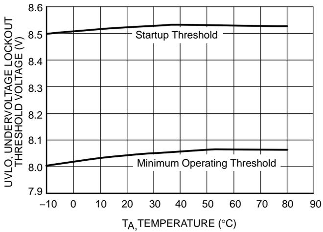
Figure 18. Undervoltage Lockout Threshold vs. Ambient Temperature
