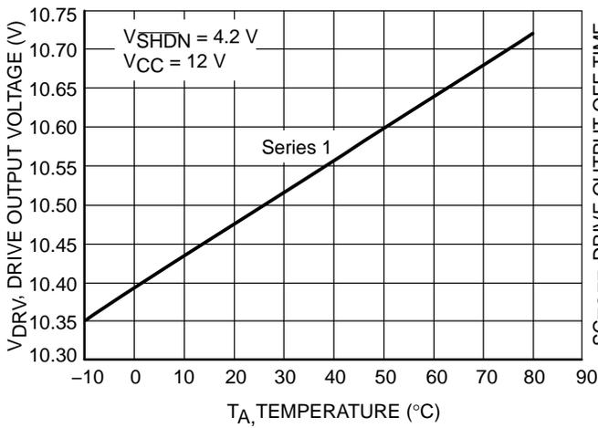
Figure 20. Regulator 2 Maximum Gate Voltage vs. Ambient Temperature
