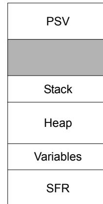
Notice that, since the stack is located immediately above the heap, using `brk()` or `sbrk()` has little effect on the size of the dynamic memory pool. The `brk()` and `sbrk()` functions are primarily intended for use in run-time environments where the stack grows downward and the heap grows upward.
