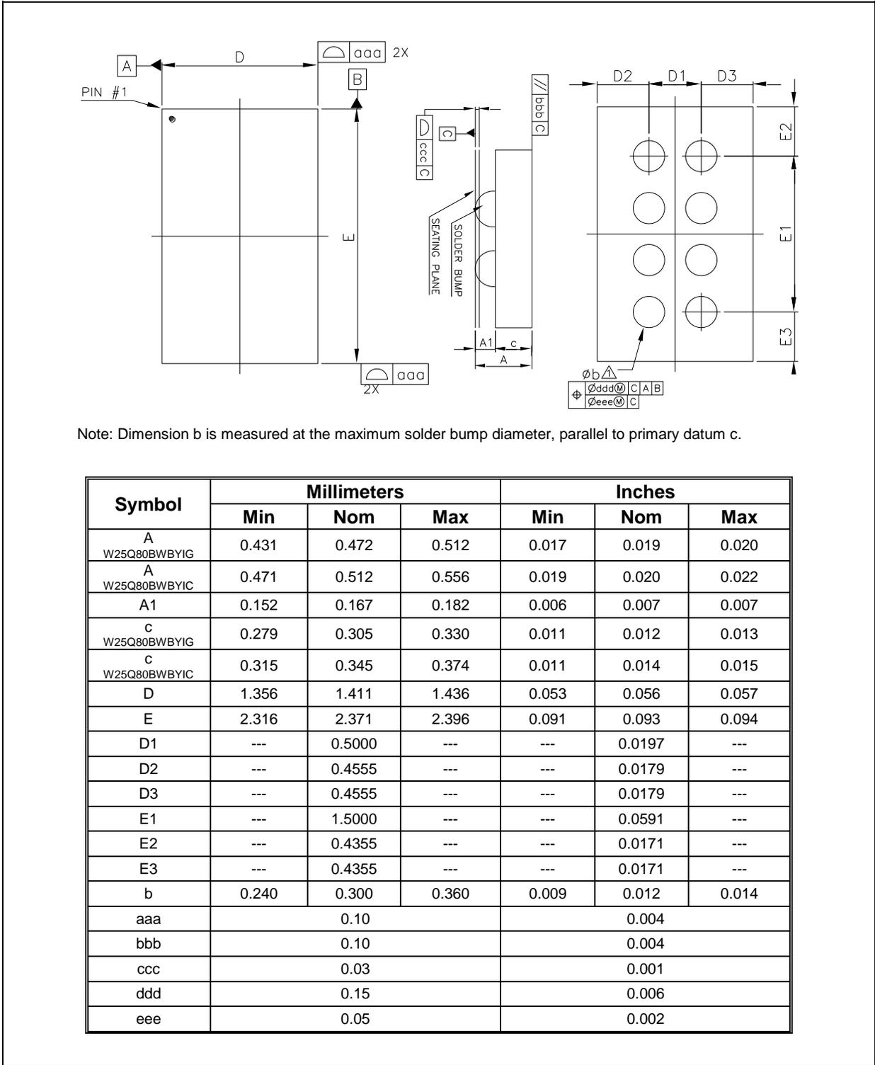
Note: Dimension b is measured at the maximum solder bump diameter, parallel to primary datum c.
