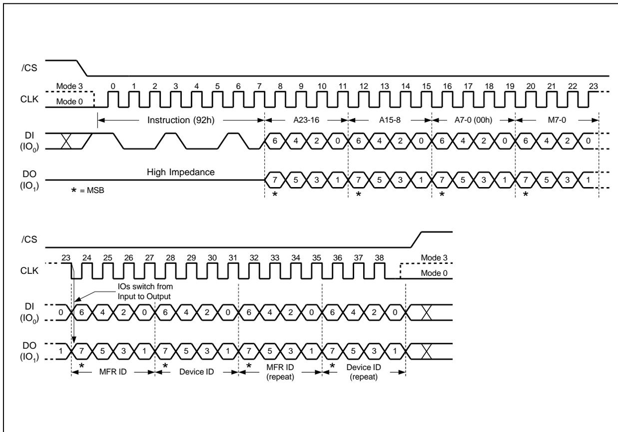
Figure 30. Read Manufacturer / Device ID Dual I/O Diagram
