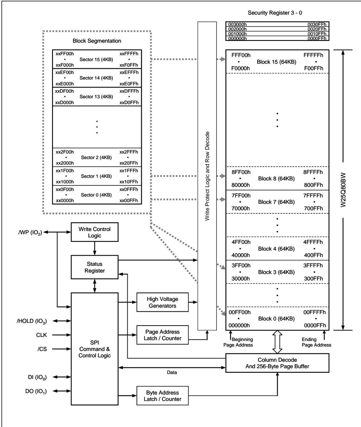
Figure 2. W25Q80BW Serial Flash Memory Block Diagram
