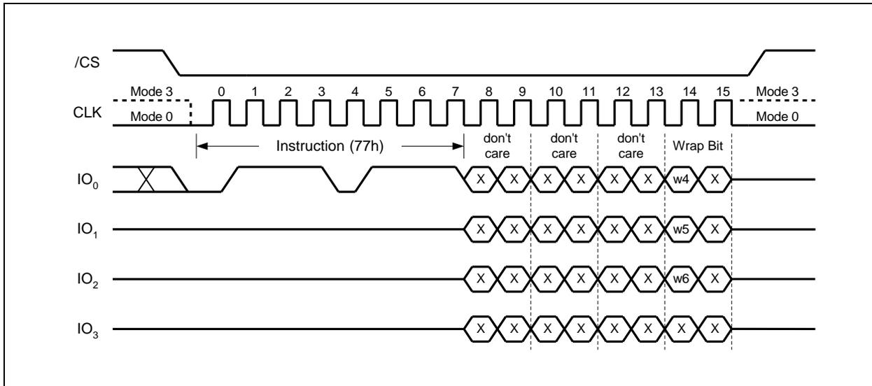
Figure 17. Set Burst with Wrap Instruction Sequence
