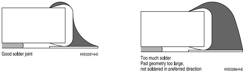
Good and poor solder joints caused by amount of solder in dual-wave soldering.
