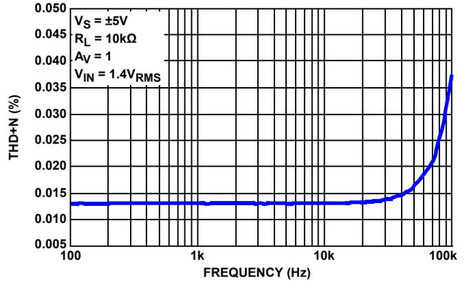
FIGURE 22. TOTAL HARMONIC DISTORTION + NOISE vs FREQUENCY
