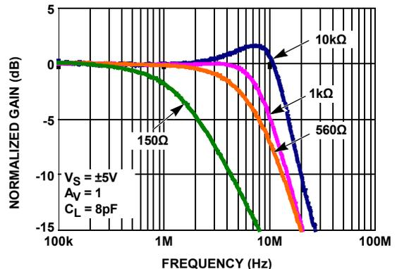
FIGURE 2. FREQUENCY RESPONSE FOR VARIOUS R<sub>L</sub>
