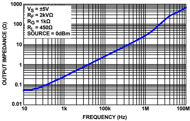
FIGURE 17. CLOSED LOOP OUTPUT IMPEDANCE vs FREQUENCY
