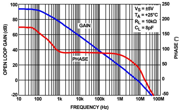
FIGURE 14. OPEN LOOP GAIN AND PHASE vs FREQUENCY
