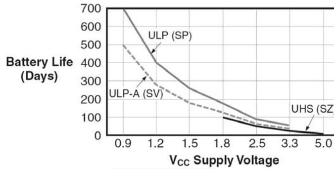
**Figure 1. Battery Life vs. V<sub>CC</sub> Supply Voltage**
