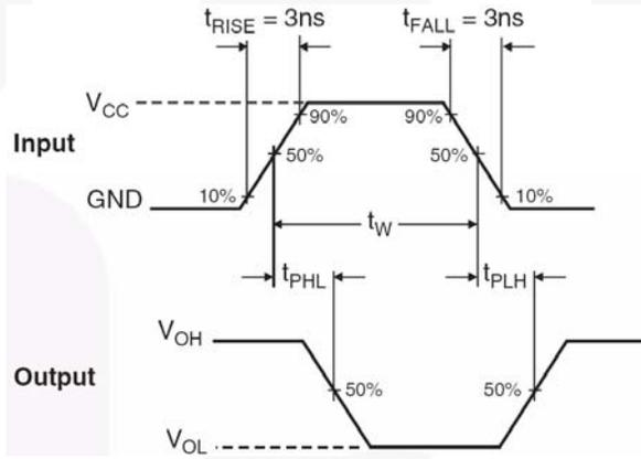
Figure 6. AC Waveforms
