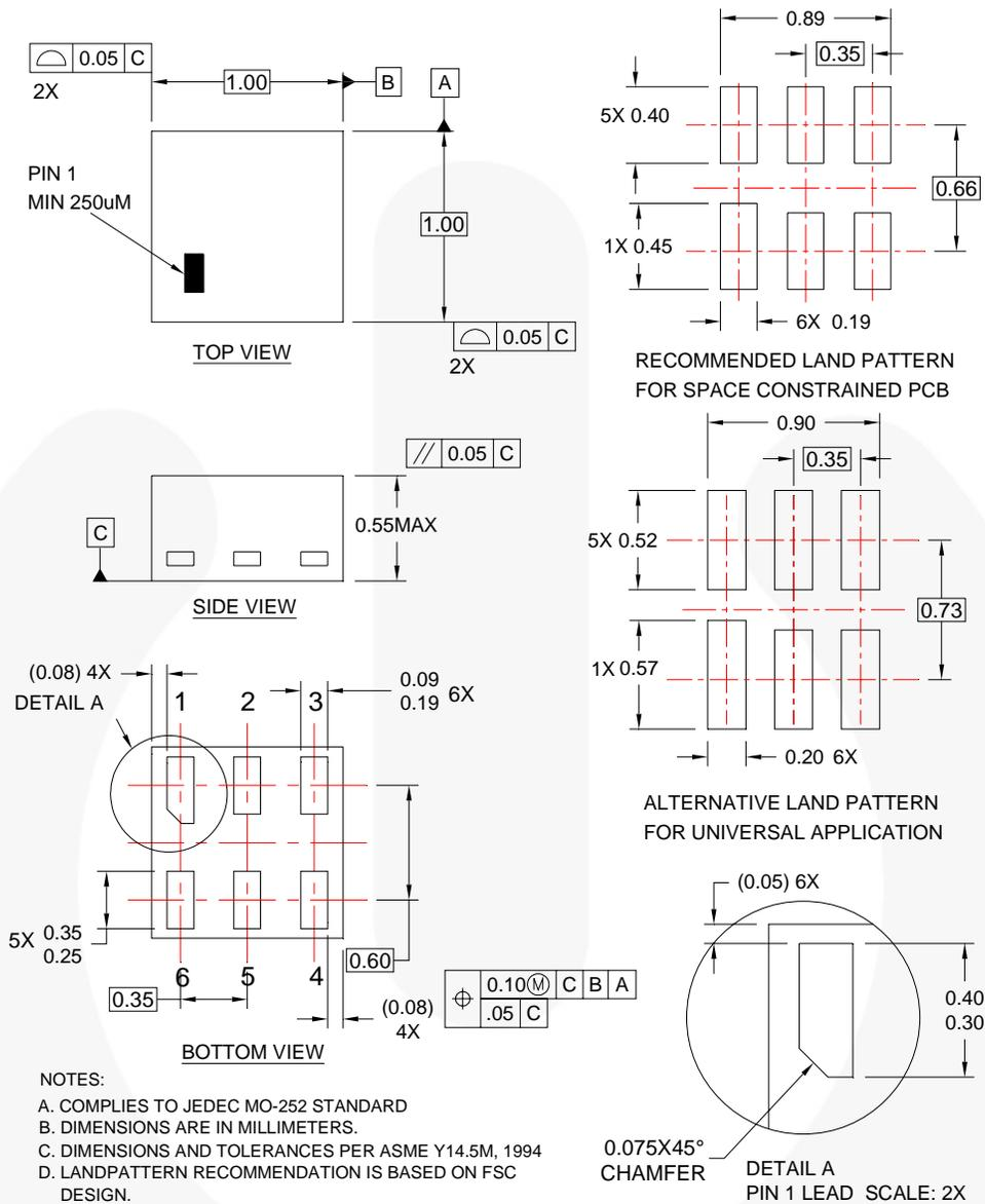
**Figure 9. 6-Lead, MicroPak2™, 1x1mm Body, .35mm Pitch**
