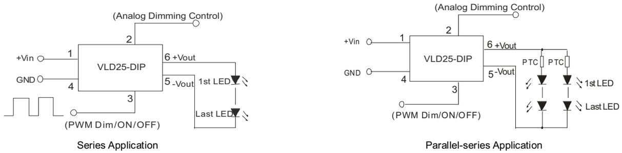
To protect the LED(s), you could connect a PTC to input of all channels as shown in application circuit.
