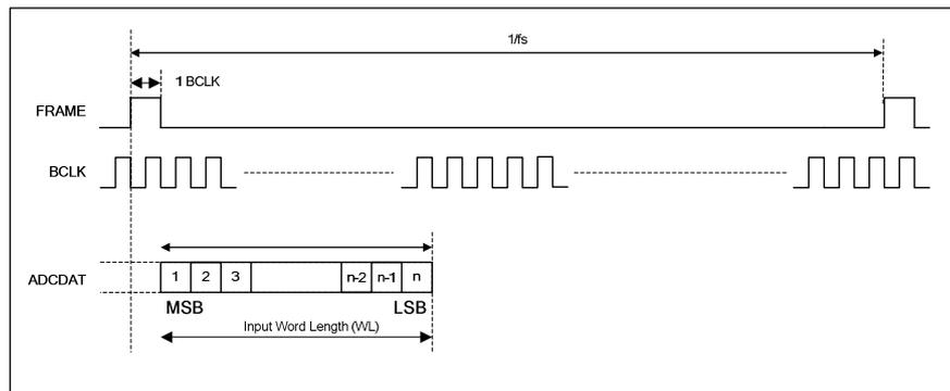
**Figure 22 DSP/PCM Mode Audio Interface (Mode A, FRAMEP=0)**
