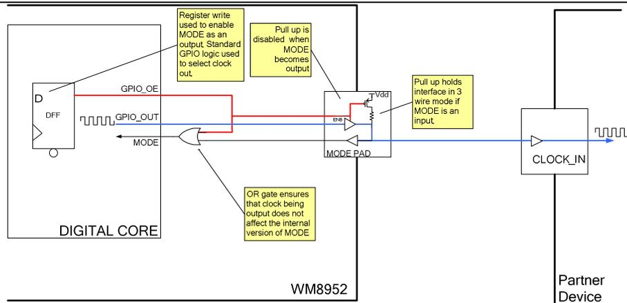
**Figure 27 Example Usage of MODE Pin to Generate a Clock Out in 3-wire Mode**
