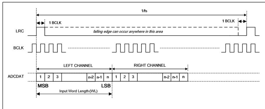
**Figure 23 DSP/PCM Mode Audio Interface (Mode B, FRAMEP=1)**
