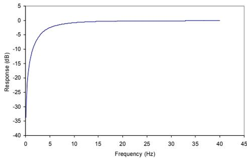
**Figure 34 ADC High Pass Filter Response, HPFAPP=0**
