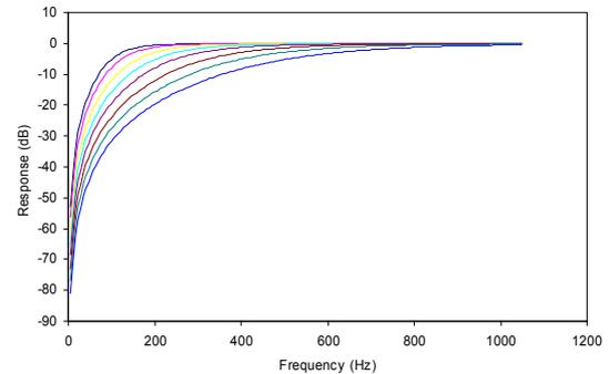
**Figure 37 ADC High Pass Filter Responses (12kHz), HPFAPP=1, all cut-off settings shown.**
