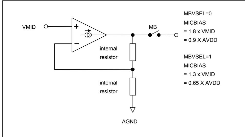
Figure 9 Microphone Bias Schematic
