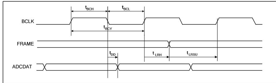
Figure 3 Digital Audio Data Timing – Slave Mode
