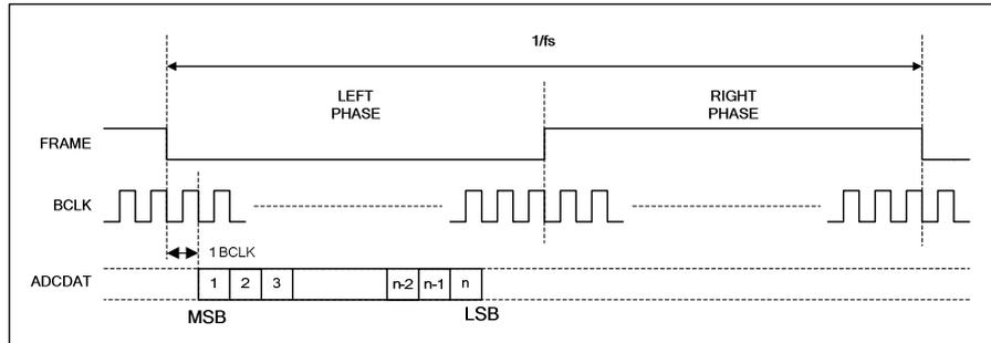
**Figure 21 I<sup>2</sup>S Audio Interface (assuming n-bit word length)**
