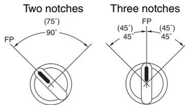
Note: 1. The angle used for automatic reset is shown in parentheses.
