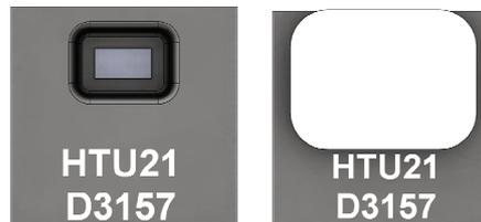
Laser marking on HTU21D(F) sensor
