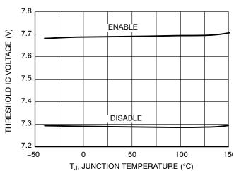
Figure 10. Threshold IC Voltage vs. Temperature
