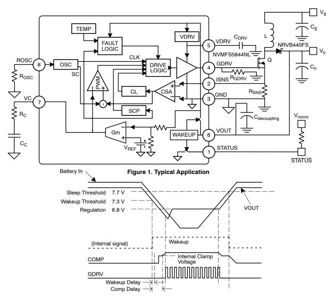
Figure 2. Functional Waveforms
