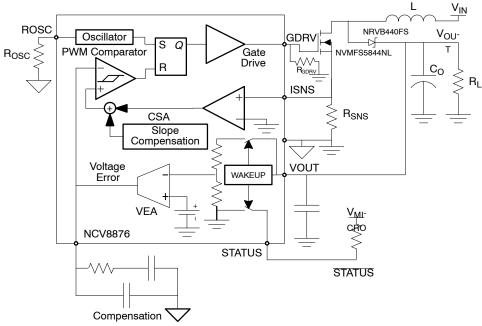
Figure 11. Current Mode Control Schematic
