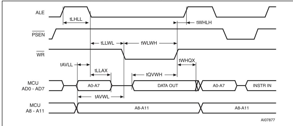
**Table 171. External WRITE cycle AC characteristics (3 V or 5 V device)**
