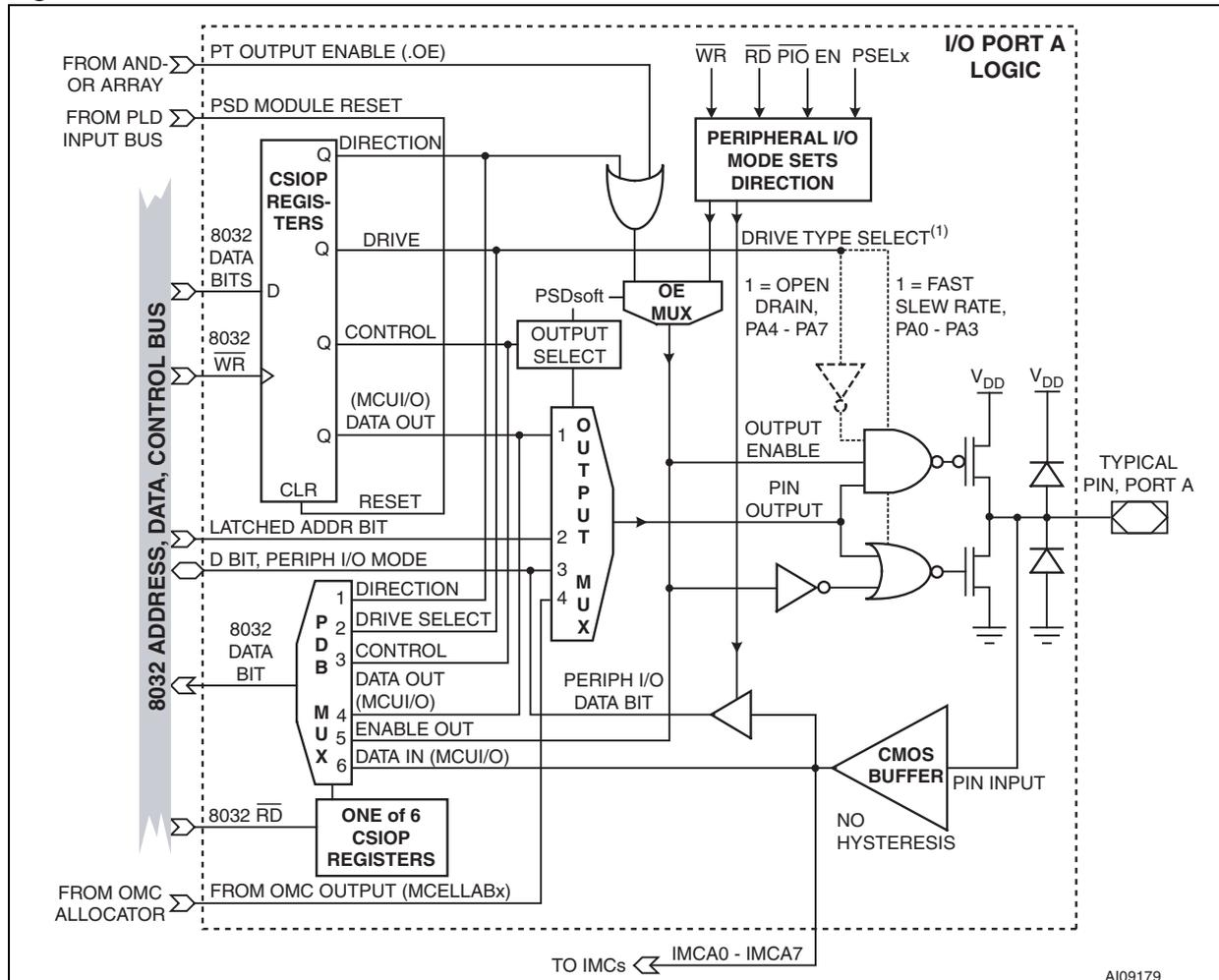
1. Port pins PA0-PA3 are capable of Fast Slew Rate output drive option. Port pins PA4-PA7 are capable of Open Drain output option.
