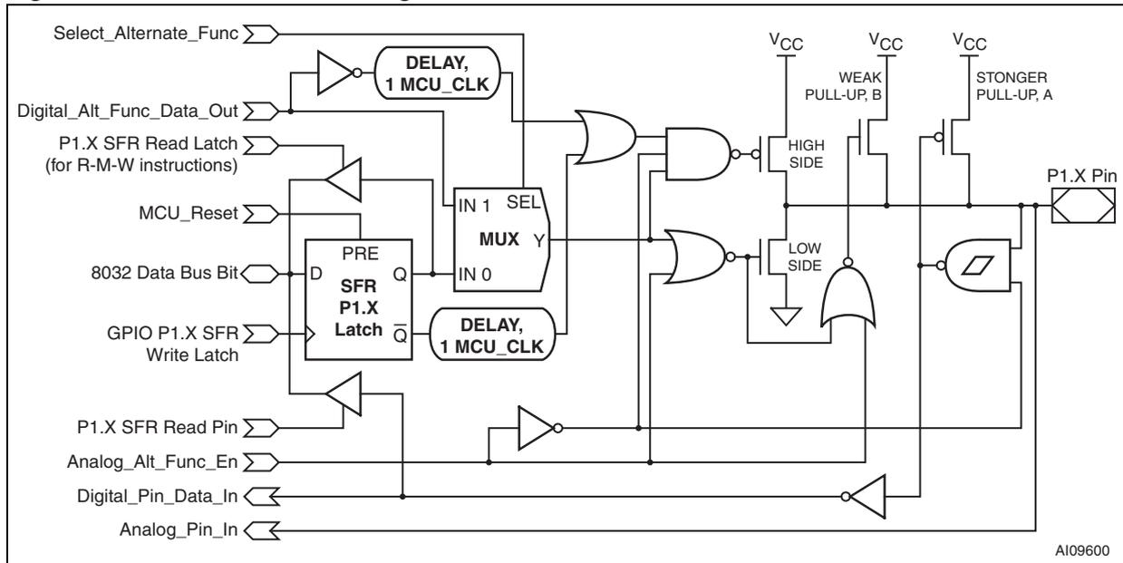
Figure 17. MCU I/O cell block diagram for Port 3
