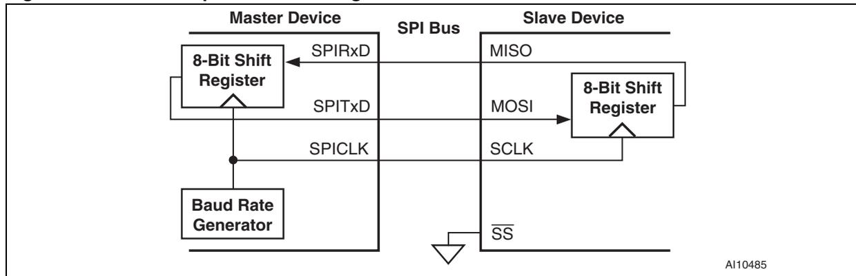
Figure 42. SPI Receive operation example
