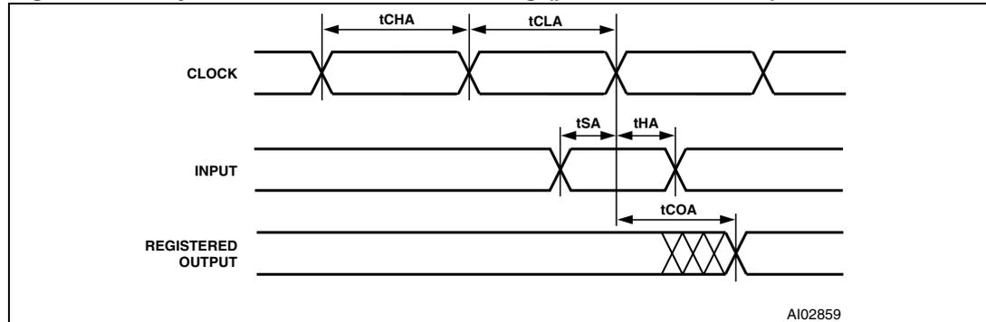
**Table 178. CPLD macrocell asynchronous Clock mode timing (5 V PSD module)**
