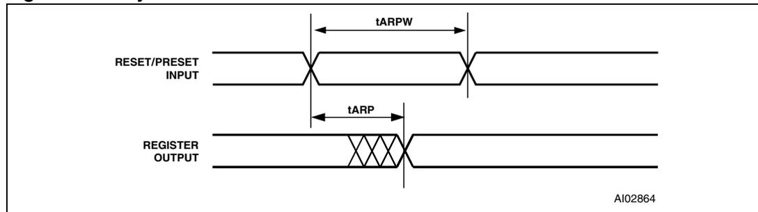
**Figure 92. Asynchronous Clock mode timing (product term clock)**
