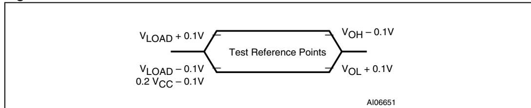
1. For timing purposes, a Port pin is considered to be no longer floating when a 100mV change from load voltage occurs, and begins to float when a 100mV change from the loaded  $V_{OH}$  or  $V_{OL}$  level occurs
