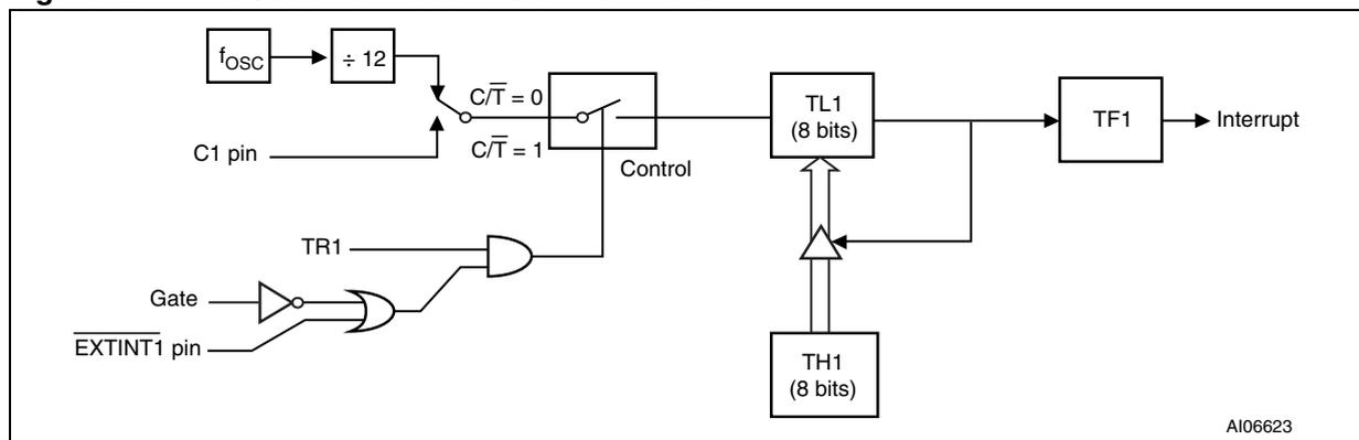
Figure 23. Timer/Counter mode 3: Two 8-bit counters
