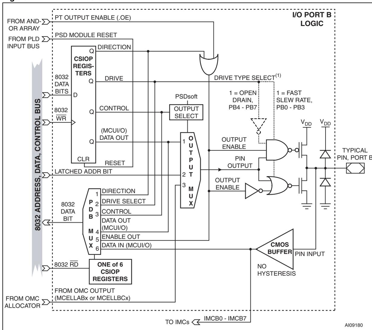
1. Port pins PB0-PB3 are capable of Fast Slew Rate output drive option. Port pins PB4-PB7 are capable of Open Drain output option.
