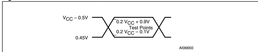
1. AC inputs during testing are driven at  $V_{CC}-0.5$  V for a logic '1,' and 0.45 V for a logic '0.'
