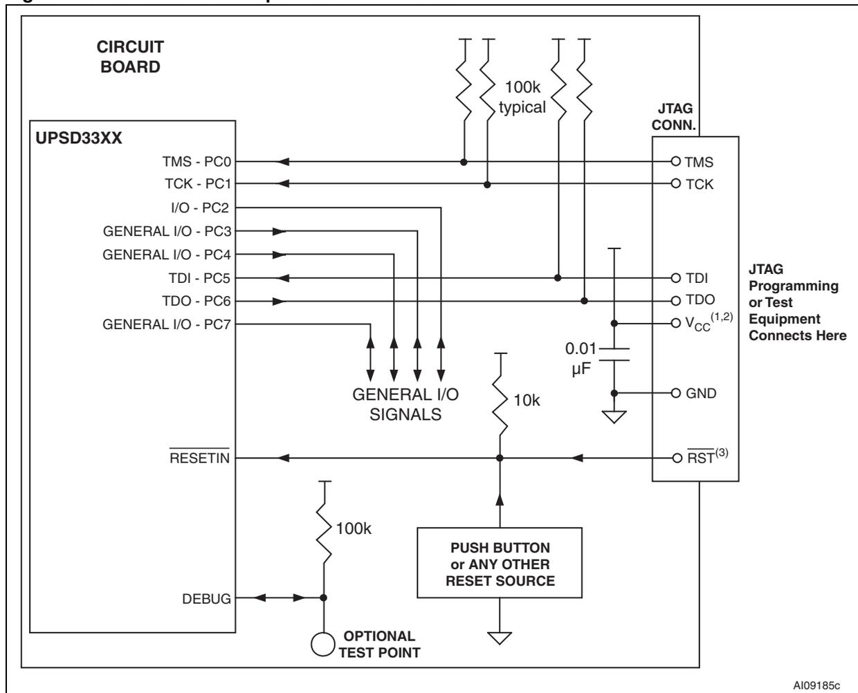
1. For 5 V UPSD33xx devices, pull-up resistors and  $V_{CC}$  pin on the JTAG connector should be connected to 5 V system  $V_{DD}$ .
