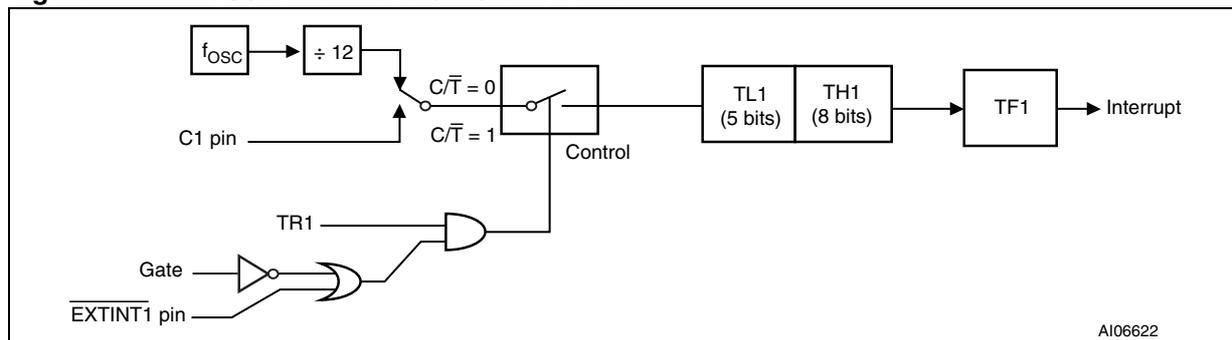
Figure 22. Timer/Counter Mode 2: 8-bit Auto-reload
