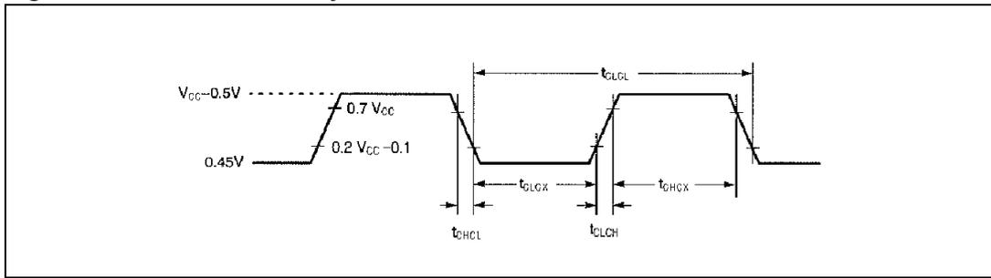
Figure 100. PSD module AC measurement I/O waveform
