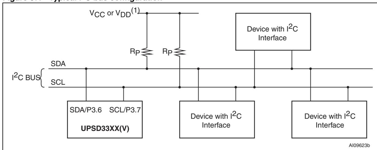
1. For 3.3 V system, connect R<sub>P</sub> to 3.3 V V<sub>CC</sub>. For 5.0 V system, connect R<sub>P</sub> to 5.0 V V<sub>DD</sub>.
