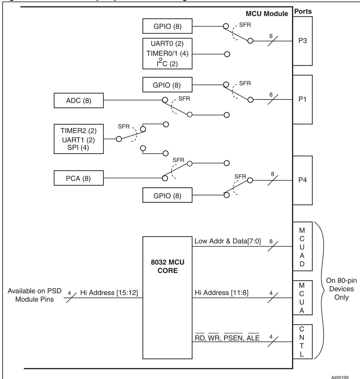
Figure 16. MCU I/O cell block diagram for Port 1
