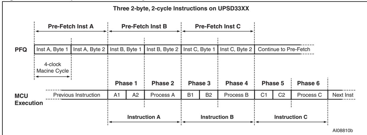
Figure 9. UPSD33xx multi-cycle instructions compared to standard 8032
