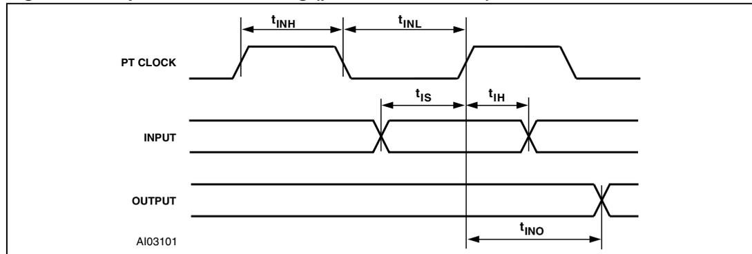
Table 180. Input macrocell timing (5 V PSD module)
