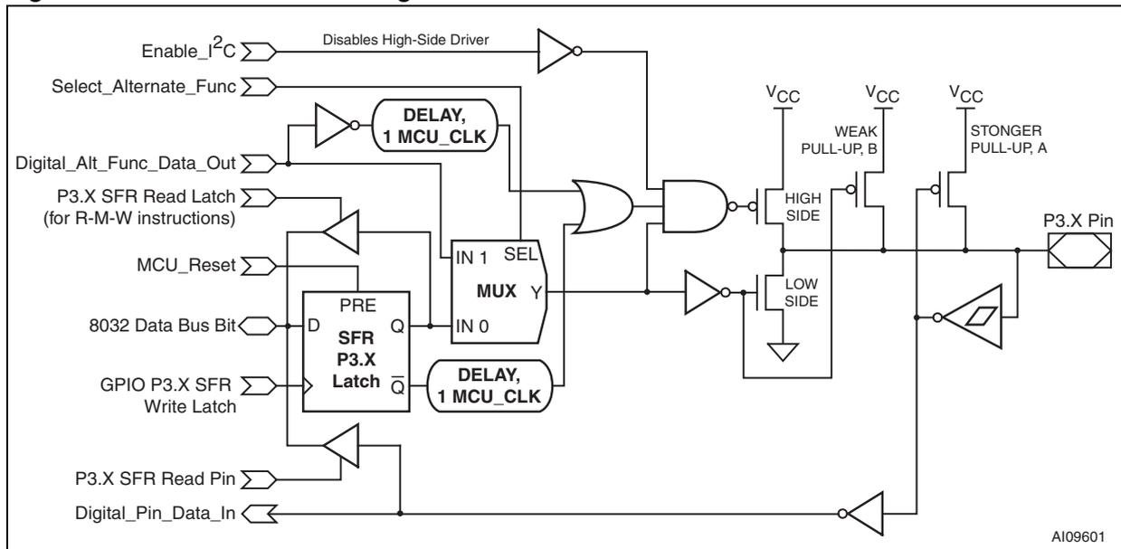
Figure 18. MCU I/O cell block diagram for Port 4
