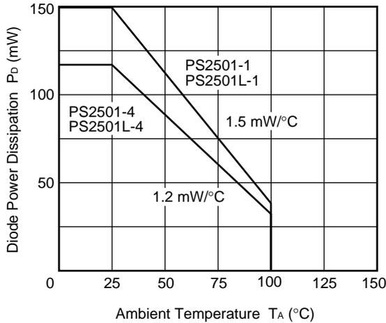
**TRANSISTOR POWER DISSIPATION vs. AMBIENT TEMPERATURE**
