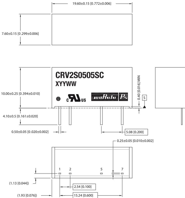
All dimensions in mm (inches) Controlling dimension is mm.
