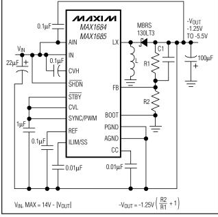
Figure 4. Inverting Output
