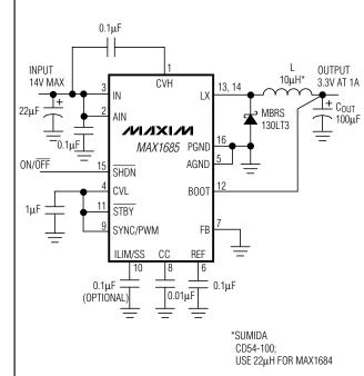
Figure 1. Standard Application Circuit
