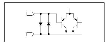
Figure 1. Input Protection Circuit
