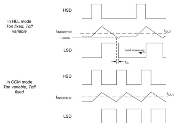
The diagram shows the signals for high side switch drive (HSD) for T<sub>ON</sub> control, the inductor current and the low side switch drive (LSD) for T<sub>OFF</sub> control.
