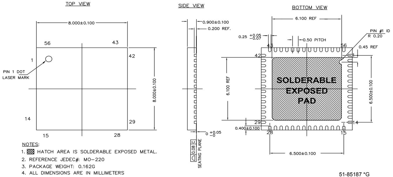
**Figure 7. 56-pin QFN 8 × 8 mm LF56A (Subcon Punch Type with 6.1 × 6.1 EPad)**
