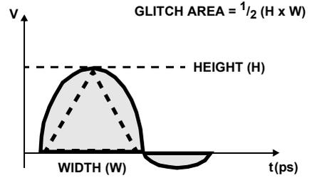
FIGURE 2. PEAK GLITCH AREA (SINGLET) MEASUREMENT METHOD
