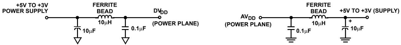
NOTE: Recommended separate analog and digital ground planes, connected at a single point near the device. See AN9827.
