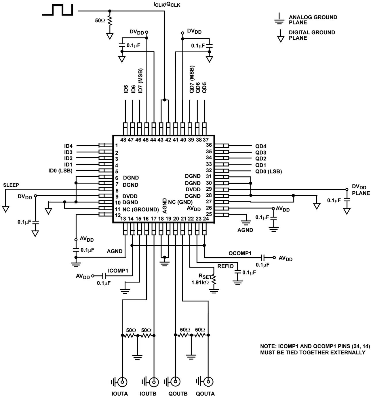
NOTE: ICOMP1 AND QCOMP1 PINS (24, 14) MUST BE TIED TOGETHER EXTERNALLY
