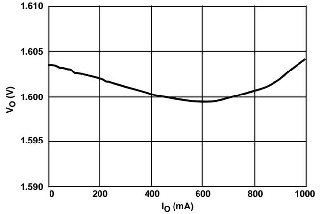
FIGURE 6. LOAD REGULATION ( $V_{IN} = 3.6V$ )
