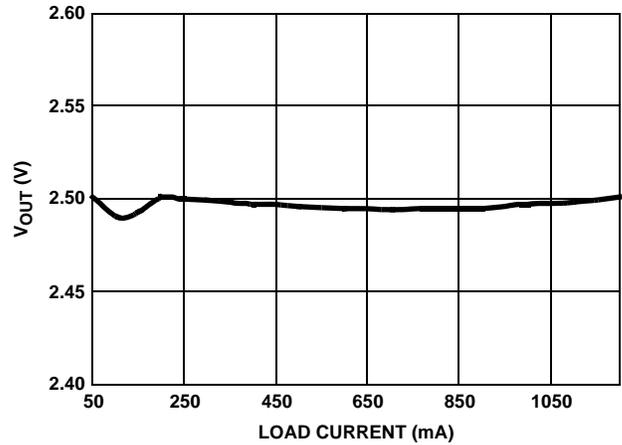
FIGURE 2.  $V_{OUT}$  vs LOAD CURRENT ( $V_{IN} = 5\text{V}$ )
