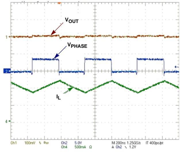
FIGURE 8. STEADY-STATE ( $V_{IN} = 3.6V$ ;  $V_O = 1.6V$ ;  $I_O = 1A$ )
