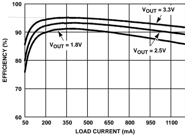
FIGURE 1. EFFICIENCY vs LOAD CURRENT ( $V_{IN} = 5.0\text{V}$ )
