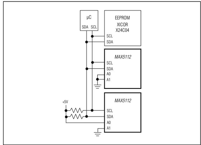
Figure 5. Typical I<sup>2</sup>C Application Circuit
