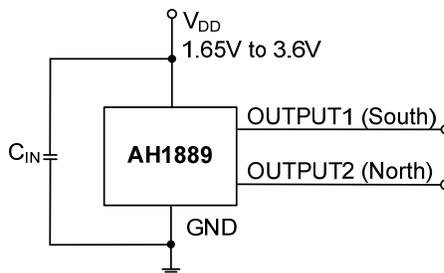
Note: 4.  $C_{IN}$  is for power stabilization and to strengthen the noise immunity, the recommended capacitance 100nF typical.
