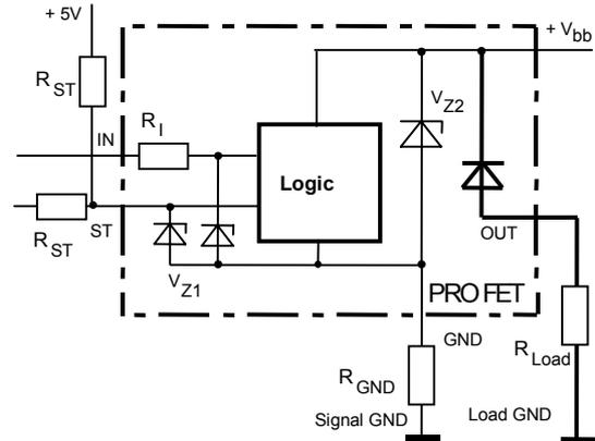
$V_{Z1} = 6.1 \text{ V typ.}$ ,  $V_{Z2} = 47 \text{ V typ.}$ ,  $R_{GND} = 150 \Omega$ ,  $R_{ST} = 15 \text{ k}\Omega$ ,  $R_I = 3.5 \text{ k}\Omega \text{ typ.}$
