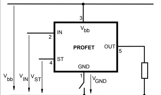
Any kind of load. In case of Input=high is  $V_{OUT} \approx V_{IN} - V_{IN(T+)}$ . Due to  $V_{GND} > 0$ , no  $V_{ST} = \text{low}$  signal available.
