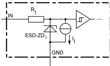
The use of ESD zener diodes as voltage clamp at DC conditions is not recommended
