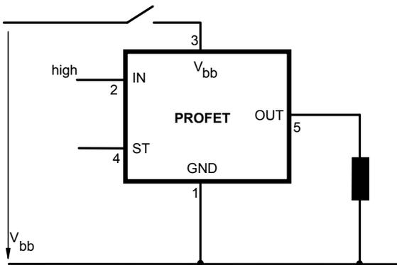
For inductive load currents up to the limits defined by  $Z_L$  (max. ratings and diagram on page 8) each switch is protected against loss of  $V_{bb}$ .
