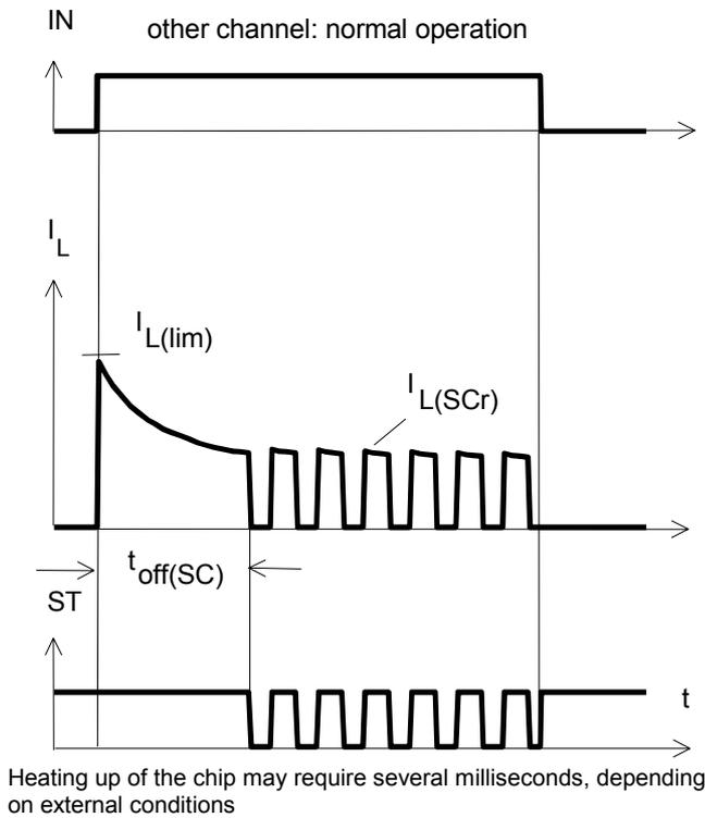
**Figure 4a:** Overtemperature: Reset if  $T_j < T_{jt}$
