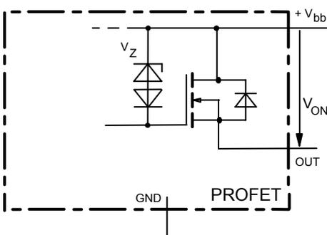
$V_{ON}$  clamped to 47 V typ.
