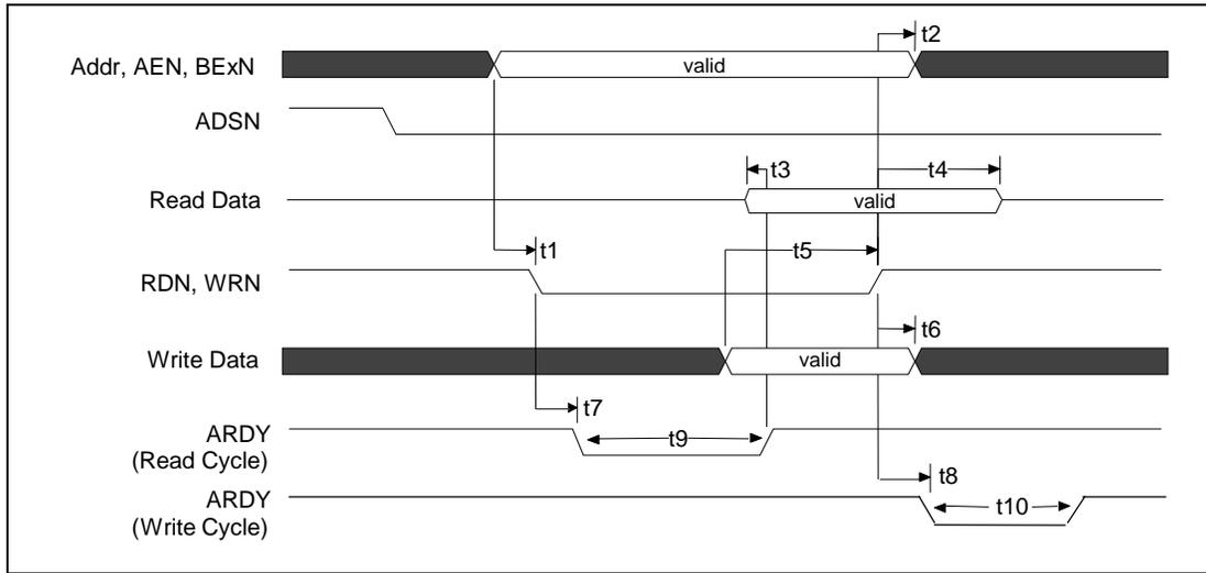
Figure 17. Asynchronous Cycle – ADSN = 0
