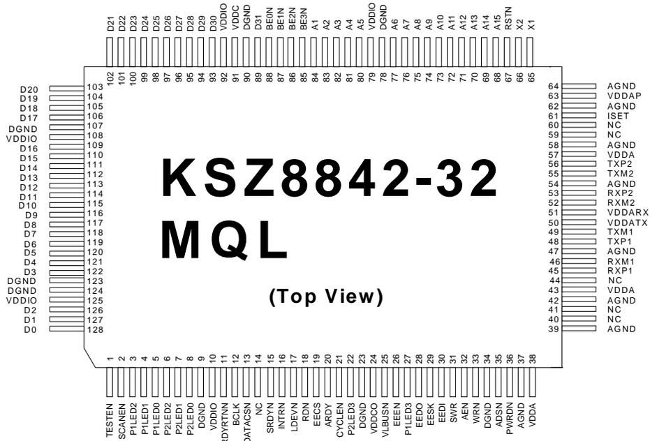
Figure 5. Standard – KSZ8842-32 MQL 128-Pin PQFP (Top View)
