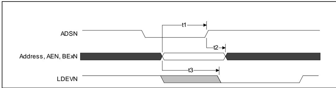
**Figure 20. Address Latching Cycle for All Modes**
