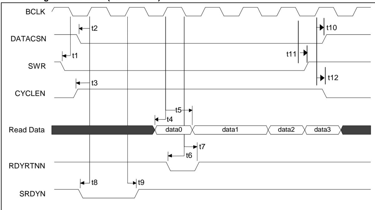
**Figure 22. Synchronous Burst Read Cycles – VLBUSN = 1**
