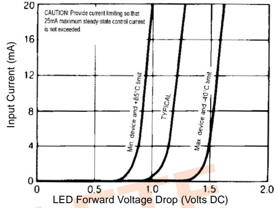
Figure 6. Input Characteristics
