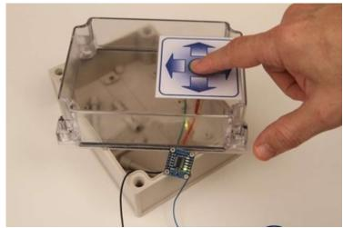
Connect the cable to the breakout. Power it up and test your control panel. Touching each button should cause a different LED to light up.
