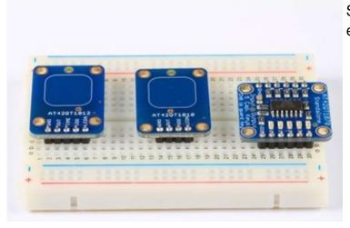
Solder each pin for solid electrical contact.
