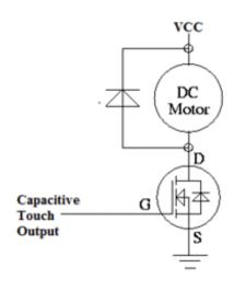
You can use it just like a pushbutton or logic signal with a transistor or MOSFET to drive high-current loads like a DC motor.
