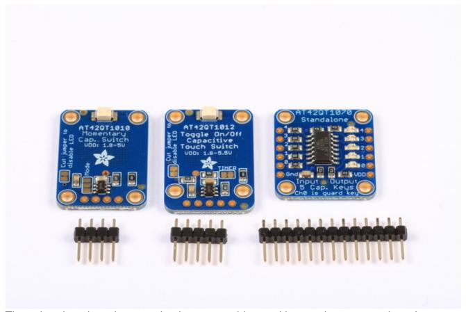
These breakout boards are a simple way to add capacitive touch to your project. Just power with 1.8 to 5.5VDC and touch the pad to activate the sensor. These touch switches interface easily to any project - with or without a microcontroller.
