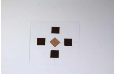
Peel the release paper from the back of the copper tape and stick the touch-pads to be back of the panel so that they align with the buttons on the front.
