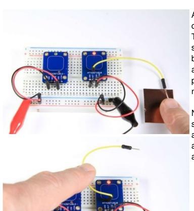
Attach the connecting wire to any conductive object or surface. That surface will become touch sensitive. Larger surfaces tend to be more sensitive. You will be able to sense through fabric, plastic glass and many other non-conductive materials.
