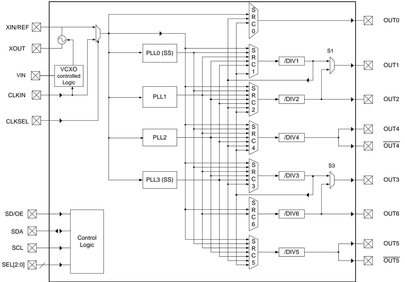
2. CLKIN, CLKSEL, SD/OE and SEL[2:0] have pull down resistors.
