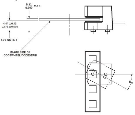
For linear motion, angular misalignment, EA, must be  $\leq \pm 2$  degrees to achieve Encoding Characteristics. All dimensions for mounting the module and codestrip should be measured with respect to the two mounting posts, shown above. Recommended Screw Size: M2.5 x 0.45 or 2-56
