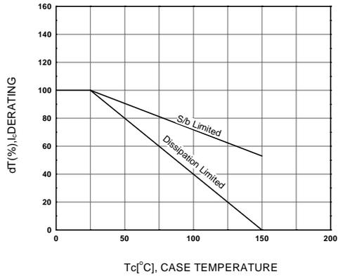
Figure 7. Derating Curve of Safe Operating Areas
