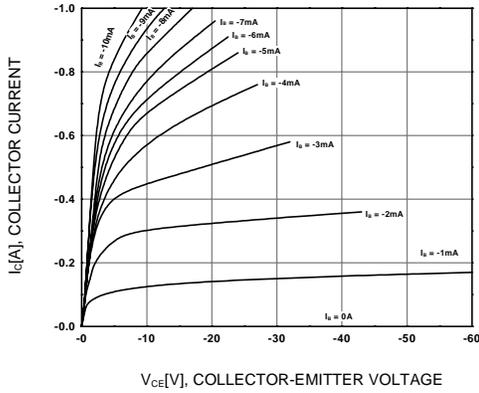
Figure 1. Static Characteristic
