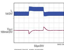
FRONT PAGE APPLICATION 1A TO 2A TRANSIENT 12V<sub>IN</sub>, 5V<sub>OUT</sub>  $C_{OUT} = 100 \mu F$
