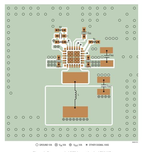
Figure 1. Recommended PCB Layout for the LT8640S
