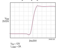
Switching Waveforms, Full **Frequency Continuous Operation**
