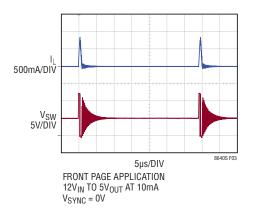
Figure 3. Burst Mode Operation
