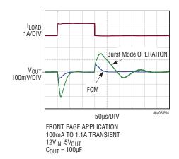
Figure 4. Load Step Transient Response with and without Forced Continuous Mode
