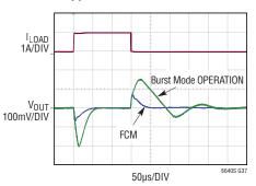
FRONT PAGE APPLICATION 100mA TO 1.1A TRANSIENT 12V<sub>IN</sub>, 5V<sub>OUT</sub> C<sub>OUT</sub> = 100μF
