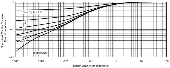
Normalized Thermal Transient Impedance, Junction-to-Foot
