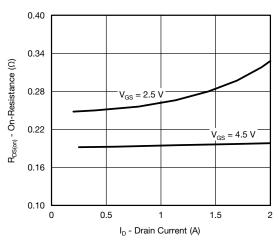
On-Resistance vs. Drain Current and Gate Voltage
