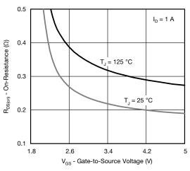
On-Resistance vs. Gate-to-Source Voltage
