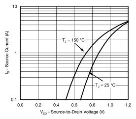
Source-Drain Diode Forward Voltage
