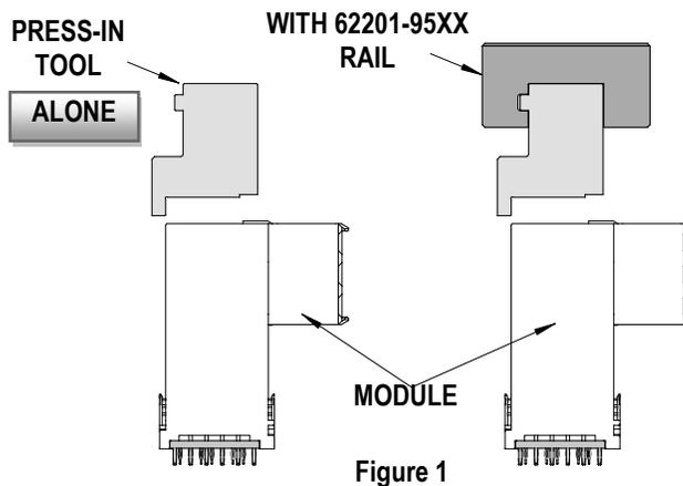
Reference: The 62203-0114 Press-In Tool is 21.5mm (0.85 in.) long.
