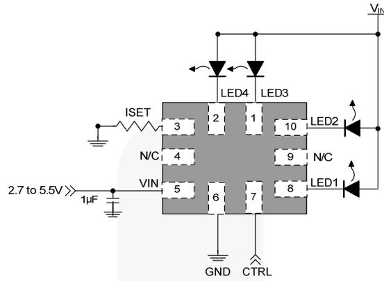
Figure 2. FAN5624 Typical Application for 4 LEDs
