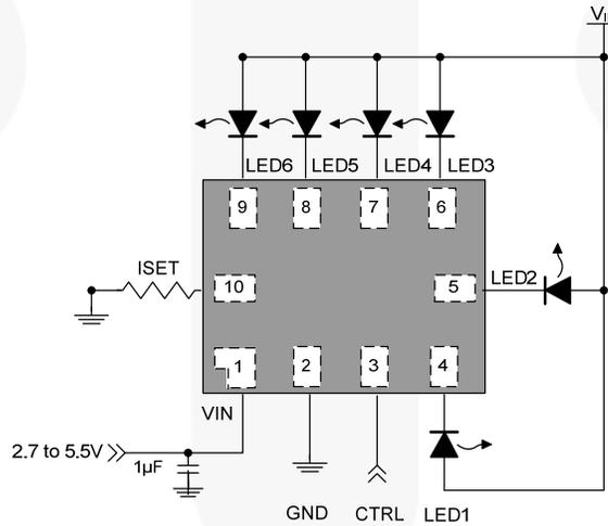
Figure 3. FAN5626 Typical Application for 6 LEDs
