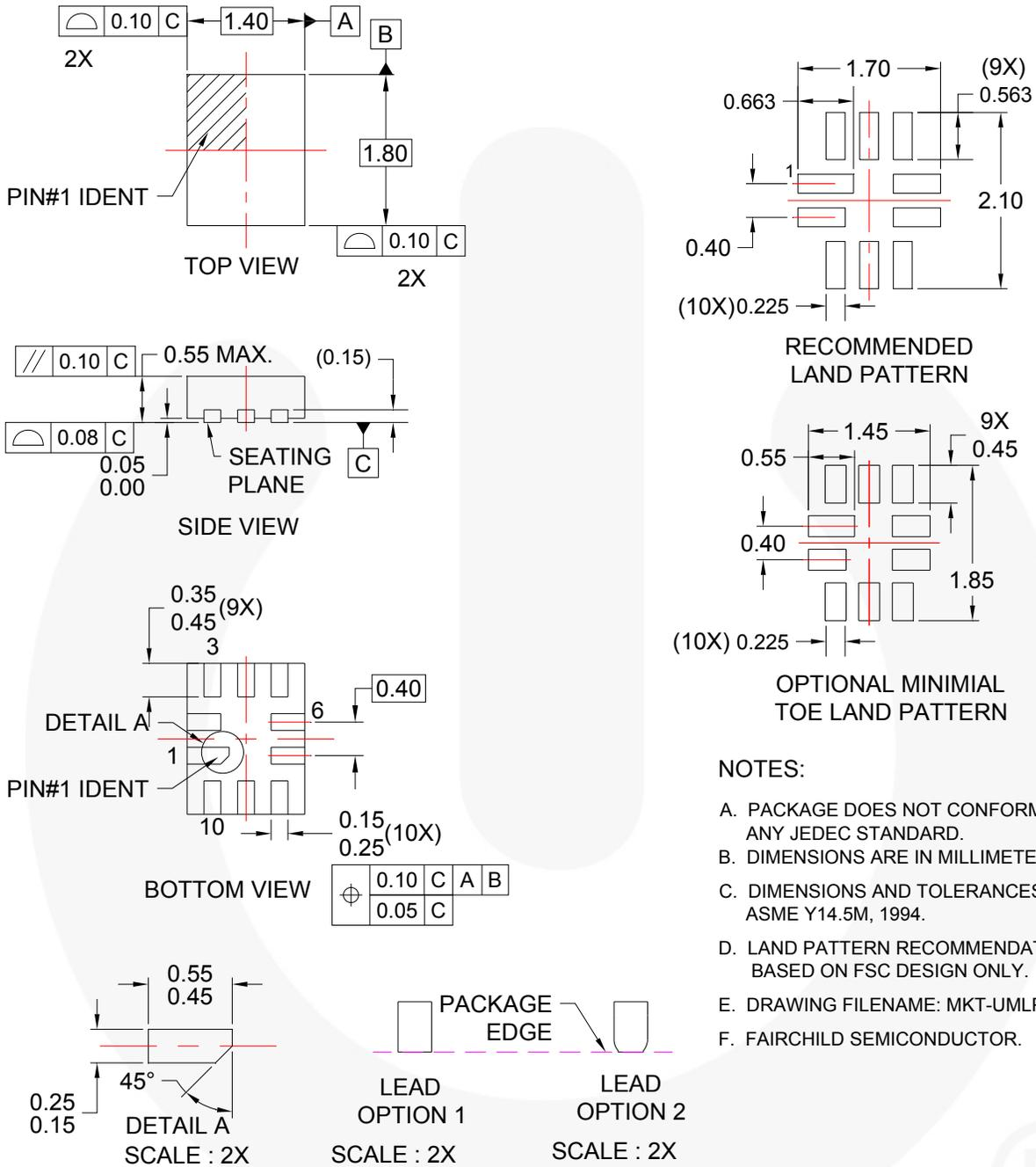
**Figure 19. 10-Lead, Ultrathin Molded Leadless Package (UMLP)**
