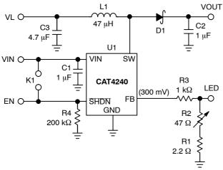
Figure 1. CAT4240AEVB Schematic
