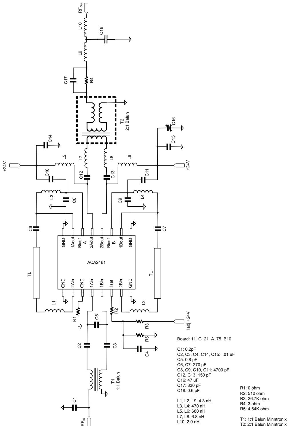
Figure 3: Application Schematic
