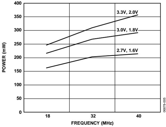
Figure 5. AFETG Power vs. Frequency (V-Driver Not Included);
