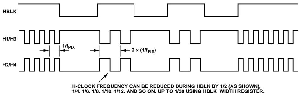
Figure 36. Generating Wide H-Clock Pulses During HBLK Interval
