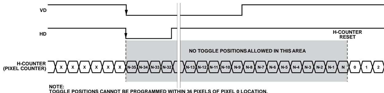
Figure 107. Toggle Position Inhibited Area, Slave Mode
