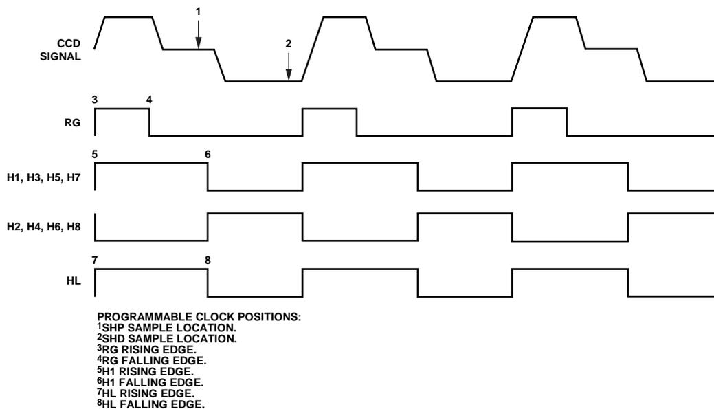
Figure 19. High Speed Clock Programmable Locations (HCLKMODE = 0x01)
