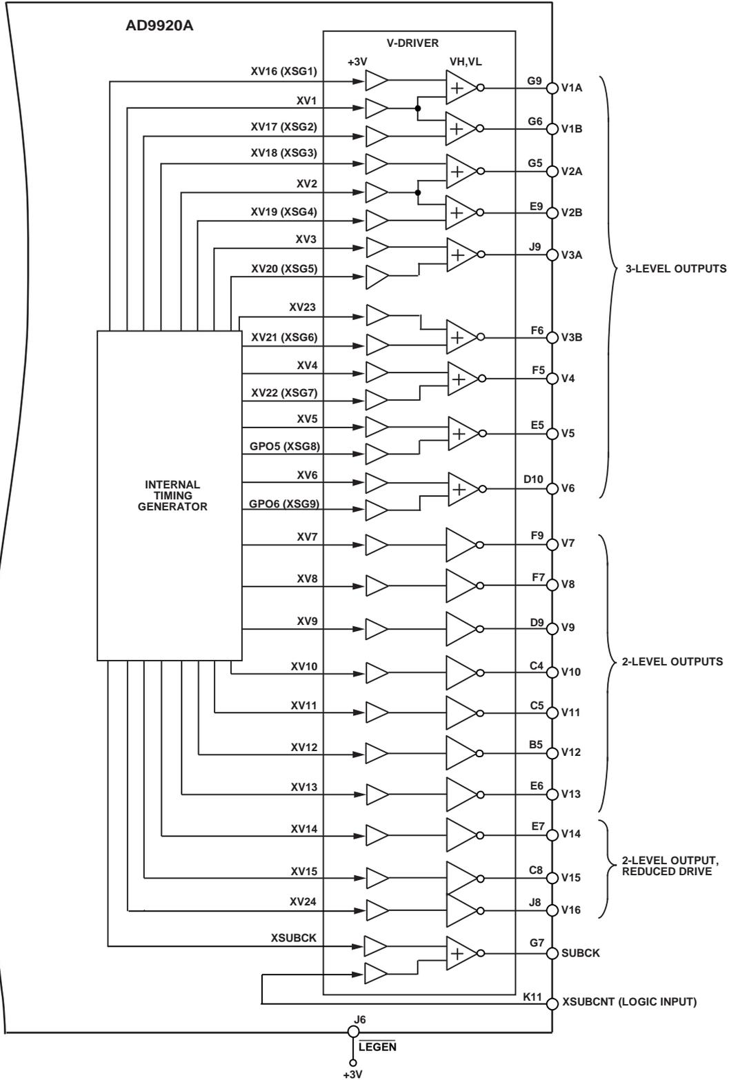
Figure 66. Internal AFETG to V-Driver Connections (19-Channel Mode)
