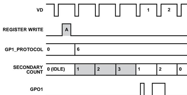
Figure 87. ShotTimer Toggle Operation Using GP\_PROTOCOL = 6
