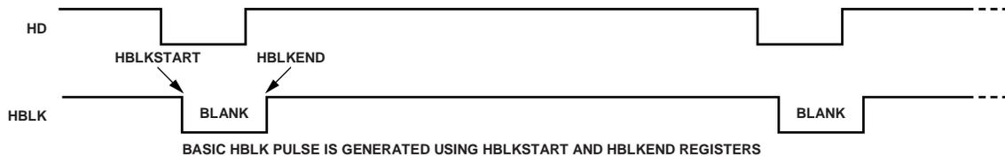
Figure 29. Typical Horizontal Blanking Pulse Placement (HBLK\_MODE = 0)
