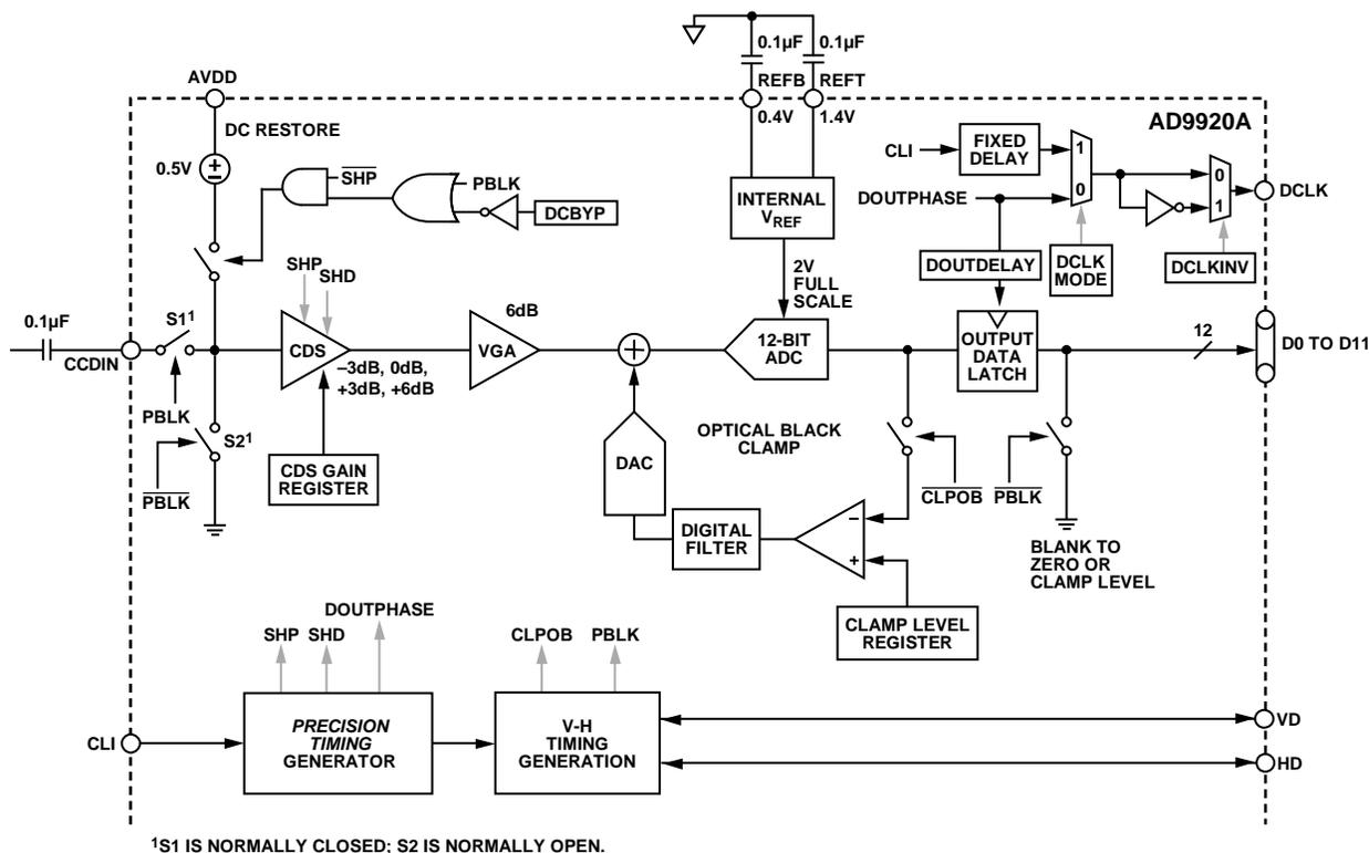
Figure 100. Analog Front End Functional Block Diagram
