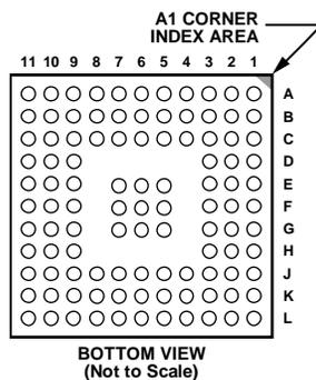
Figure 4. Pin Configuration
