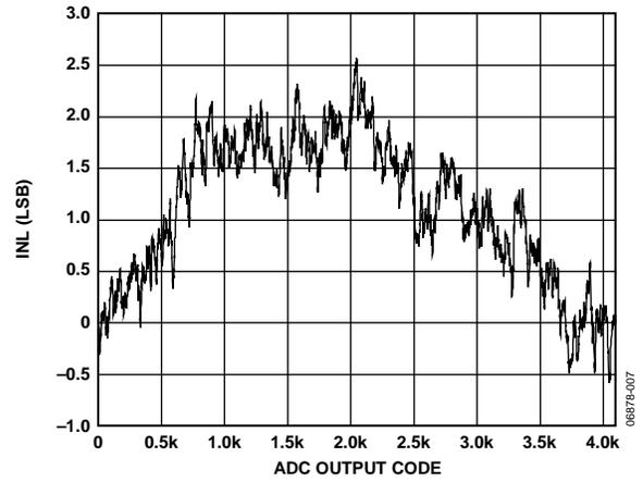
Figure 7. Typical System Integral Nonlinearity (INL) Performance
