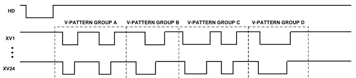
Figure 45. Combining Multiple V-Patterns Using CONCAT\_GRP = 1
