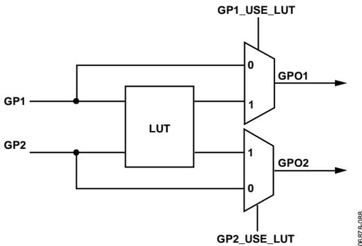
Figure 88. Internal LUT for GPO1 and GPO2 Signals
