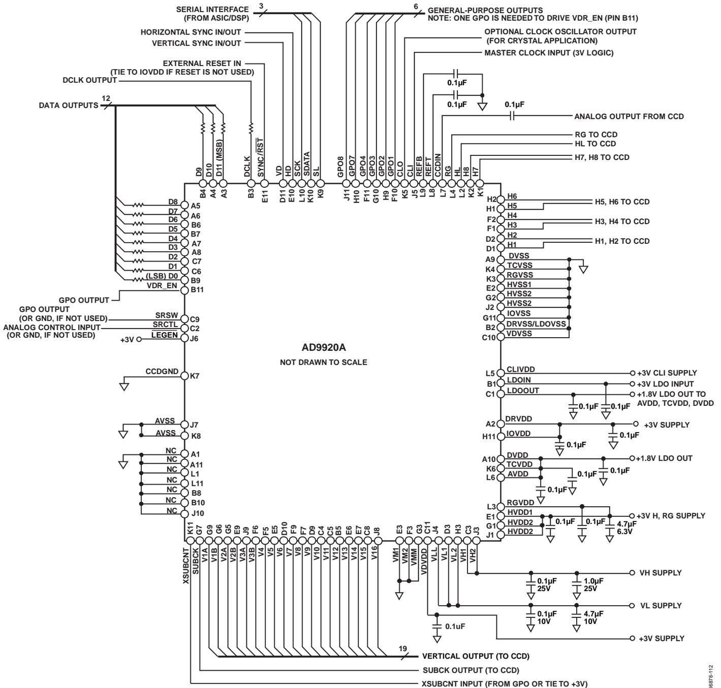
Figure 112. Typical 3V Circuit Configuration in 19-Channel Mode
