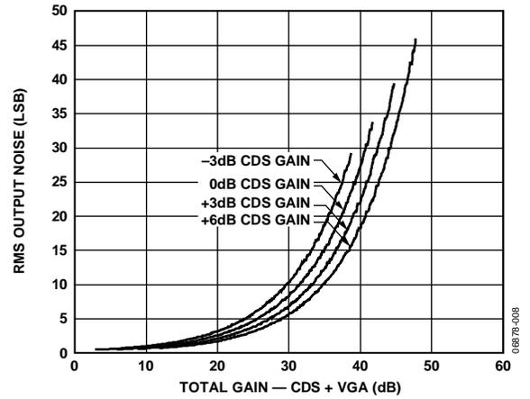
Figure 8. Output Noise vs. Total Gain (CDS + VGA)
