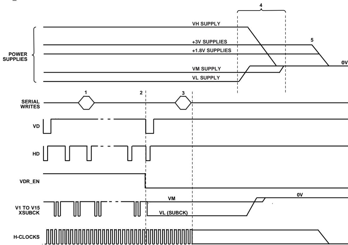
Figure 104. Recommended Power-Down Sequence, Master or Slave Mode
