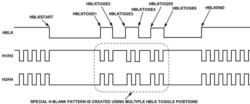
Figure 31. Using Multiple Toggle Positions for HBLK (HBLK\_MODE = 0)
