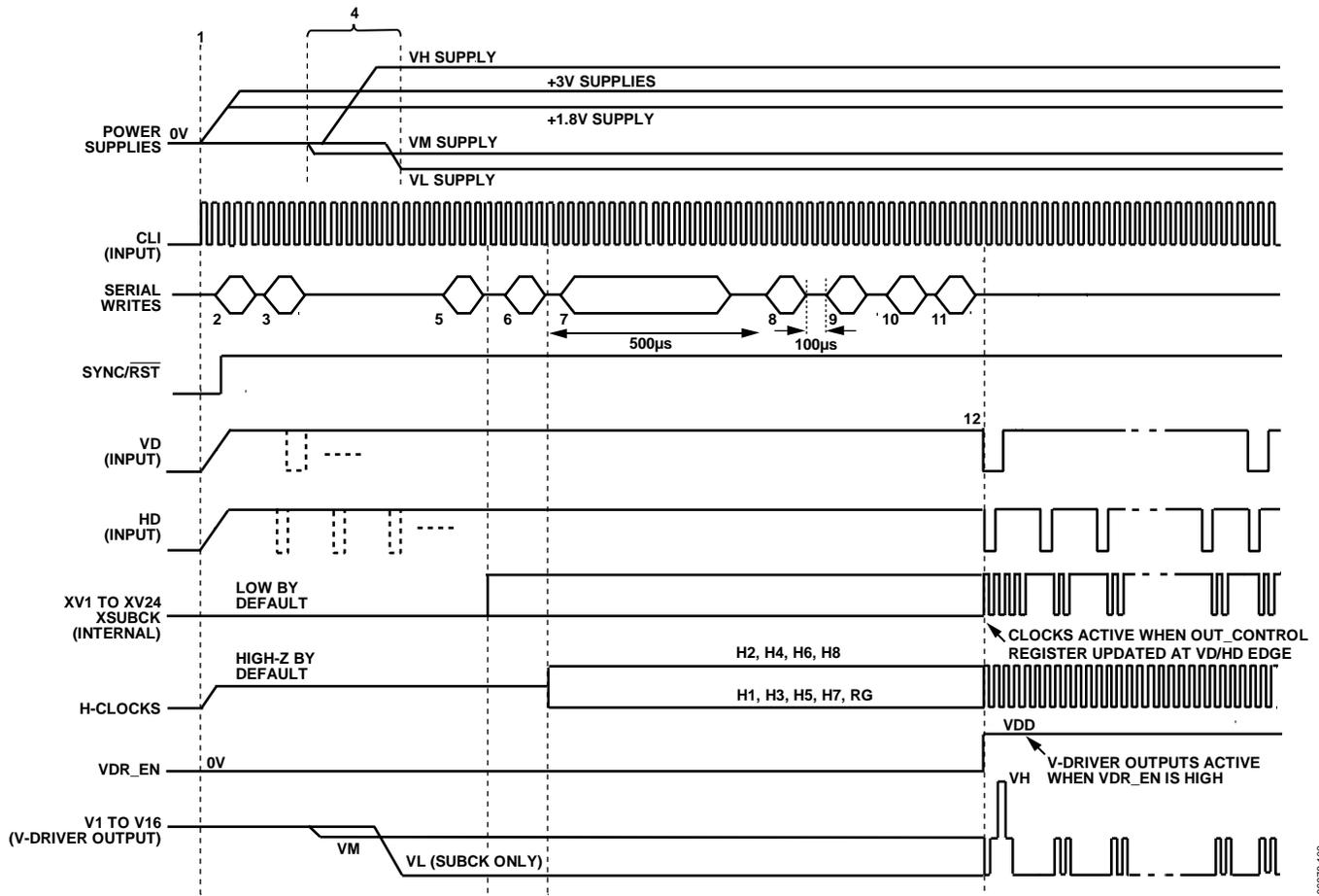
Figure 103. Recommended Power-Up Sequence and Synchronization, Slave Mode
