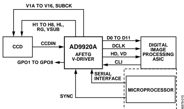
Figure 15. Typical System Block Diagram, Master Mode
