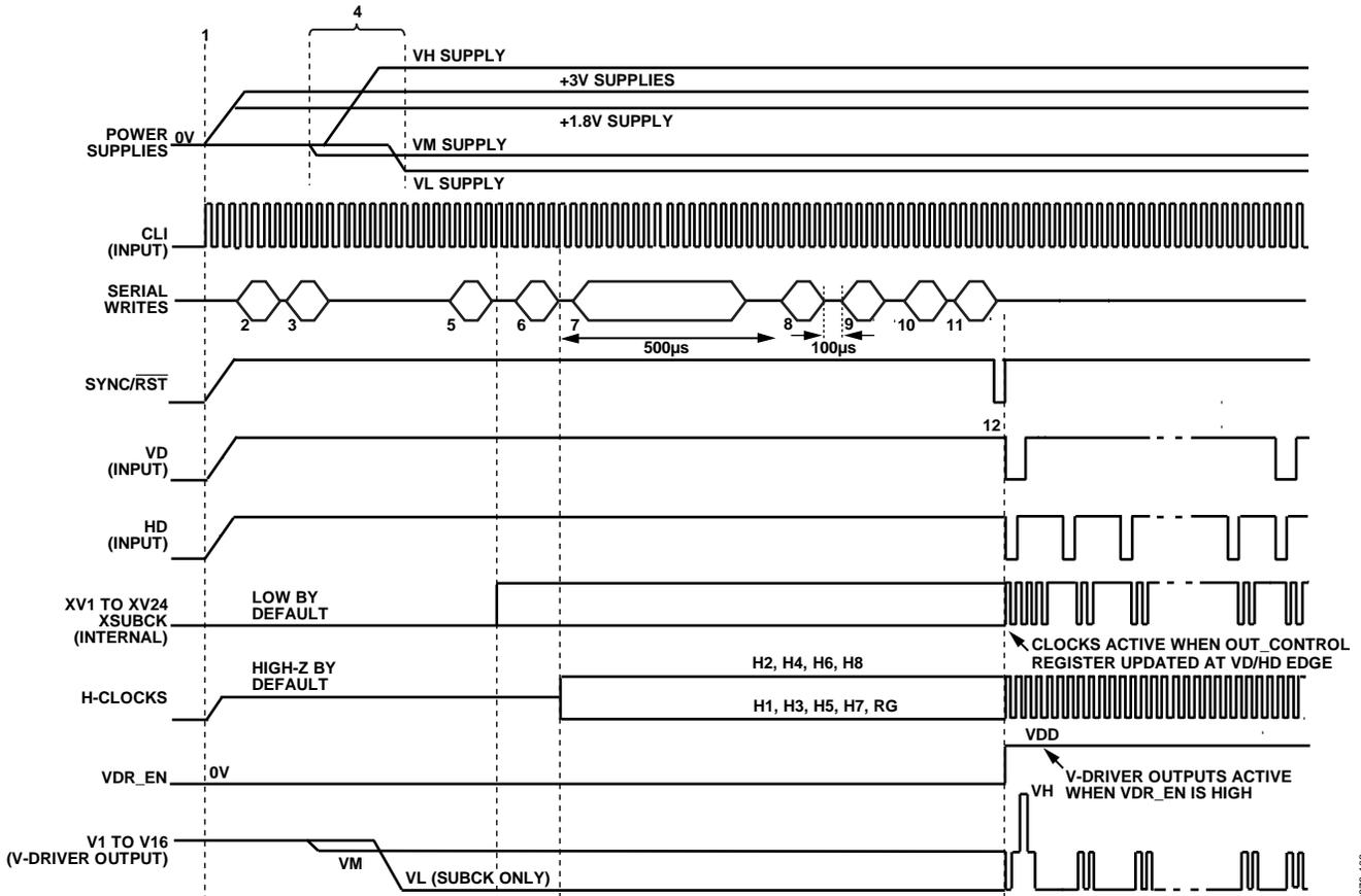
Figure 102. Recommended Power-Up Sequence and Synchronization, Master Mode
