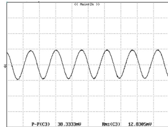
Figure 11: Output ripple & noise at 12Vin, 3.3V/10A out
