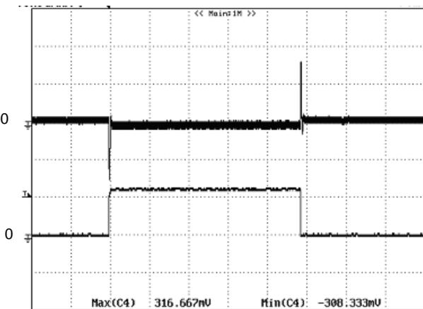
**Figure 17:** Typical transient response to step load change at
