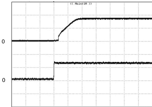
**Figure 15:** Turn on delay time at 12Vin, 3.3V/10A out
