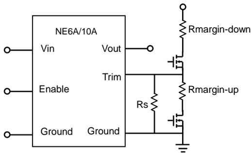
**Figure 22:** Circuit configuration for output voltage margining
