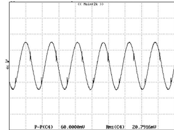
Figure 12: Output ripple & noise at 12Vin, 5.0V/10A out
