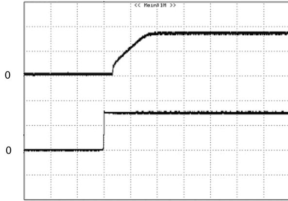
**Figure 14:** Turn on delay time Remote On/Off, 1.0V/10A out
