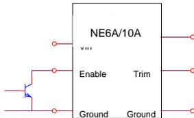
**Figure 19:** Enable Input drive circuit for NE series
