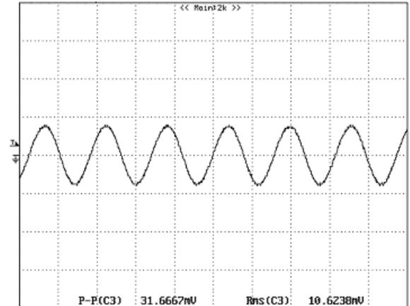
Figure 10: Output ripple & noise at 12Vin, 2.5V/10A out
