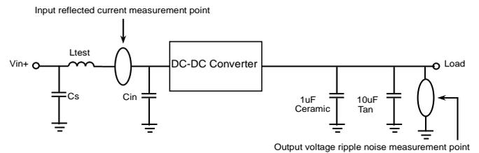
$$C_s = 270\mu\text{F} \times 1, L_{\text{test}} = 2\mu\text{H}, C_{\text{in}} = 270\mu\text{F} \times 1$$
