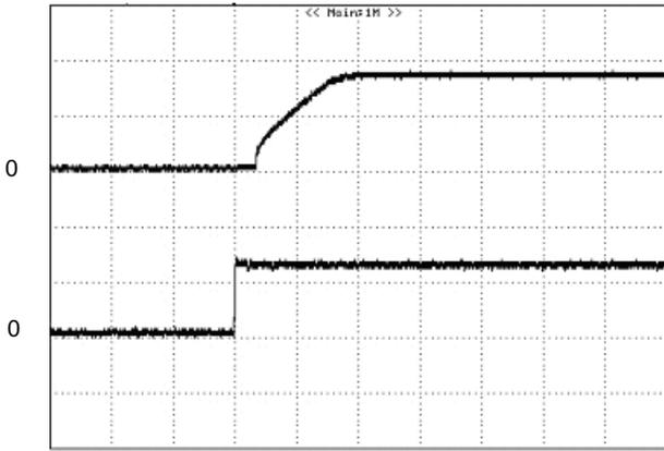
**Figure 13:** Turn on delay time at 12Vin, 1.0V/10A out
