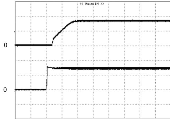
**Figure 16:** Turn on delay time at Remote On/Off, 3.3V/10A out
