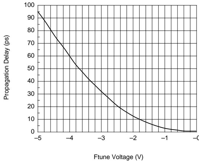
Propagation Delay vs Ftune Voltage (10E196)
