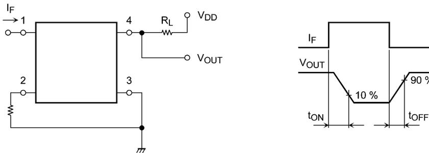
**Fig. 11.1 Switching Time Test Circuit and Waveform**
