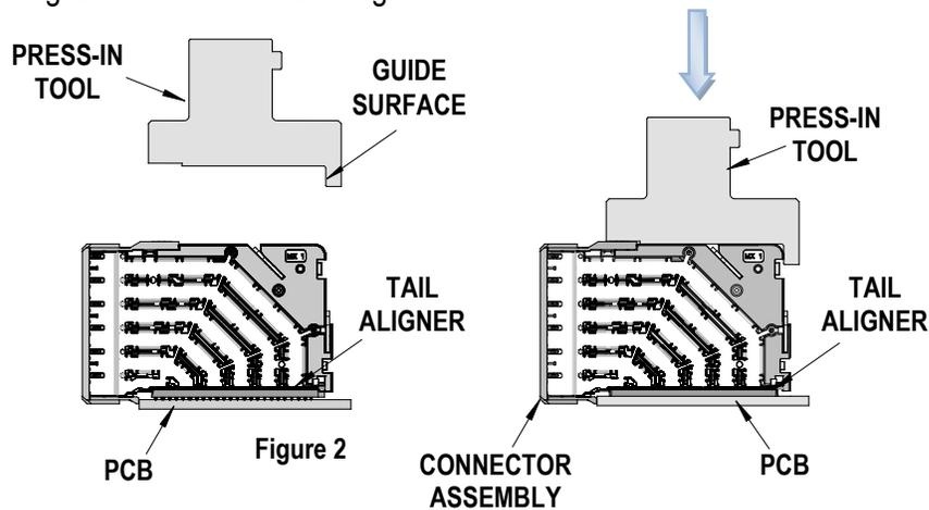
3. Using the application tool and an appropriate press, seat the Daughtercard module until there is less than 0.10mm (.004) in clearance between the bottom of the aligner and the surface of the PCB. See Figure 3.
