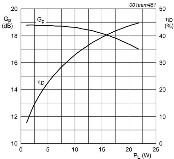
$V_{DS} = 28$  V;  $I_{Dq} = 345$  mA;  $f = 2140$  MHz.
