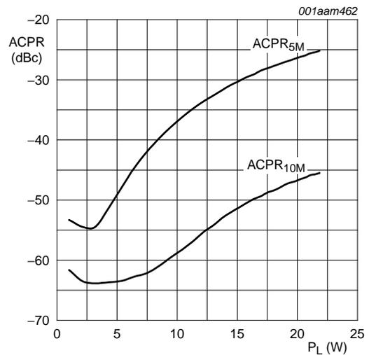
$V_{DS} = 28$  V;  $I_{Dq} = 345$  mA;  $f = 2140$  MHz.
